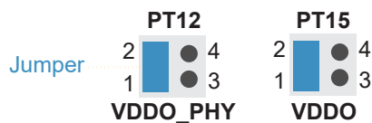
Figure 10: Connect Pins 1 and 2 on PT12 and PT15
