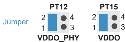
Figure 6: Connect Pins 1 and 2 on PT12 and PT15
