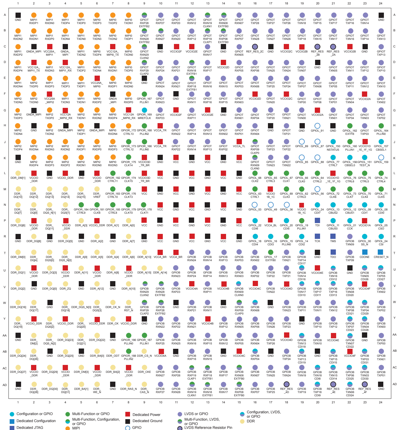
Figure 39: 576-Ball FBGA Pinout Diagram
