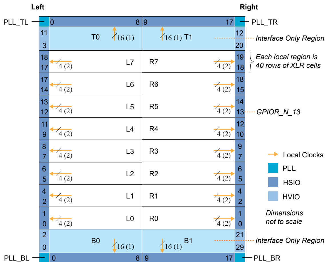
Figure 14: Clock Sources that Drive the Interfaces
