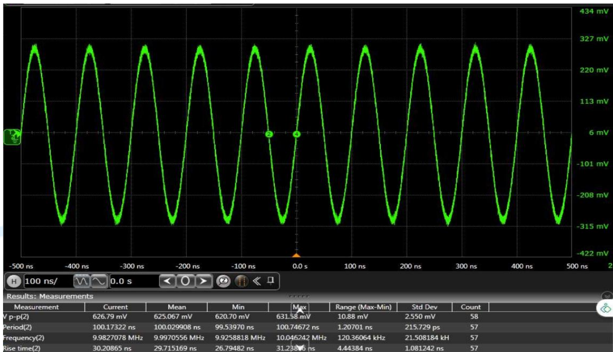
Figure 4: Time domain 10 MHz output waveform for x8 interpolation, LMF = 244 mode
