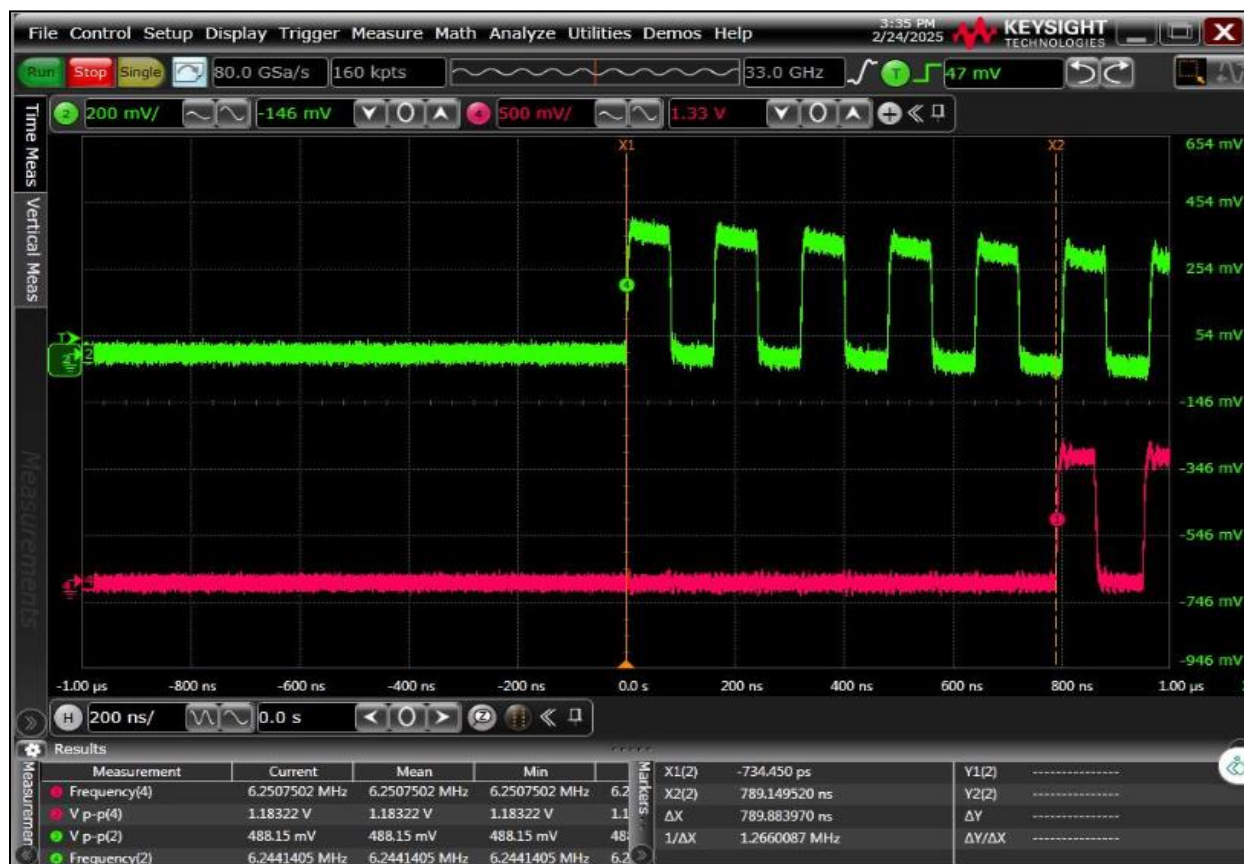
Figure 7: Deterministic Latency capture between reference square pulse(green) and ADC samples MSB output(pink).
