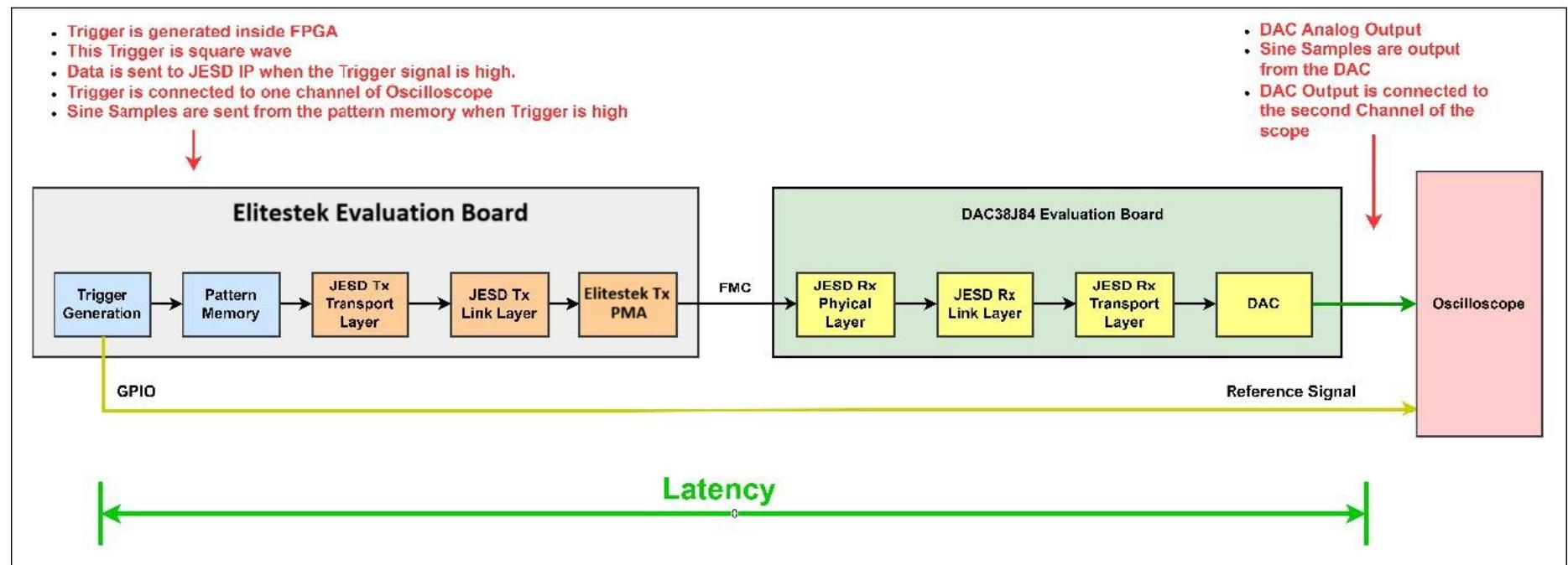
Figure 83. Deterministic Latency testing of JESD204B Transmitter with DAC
