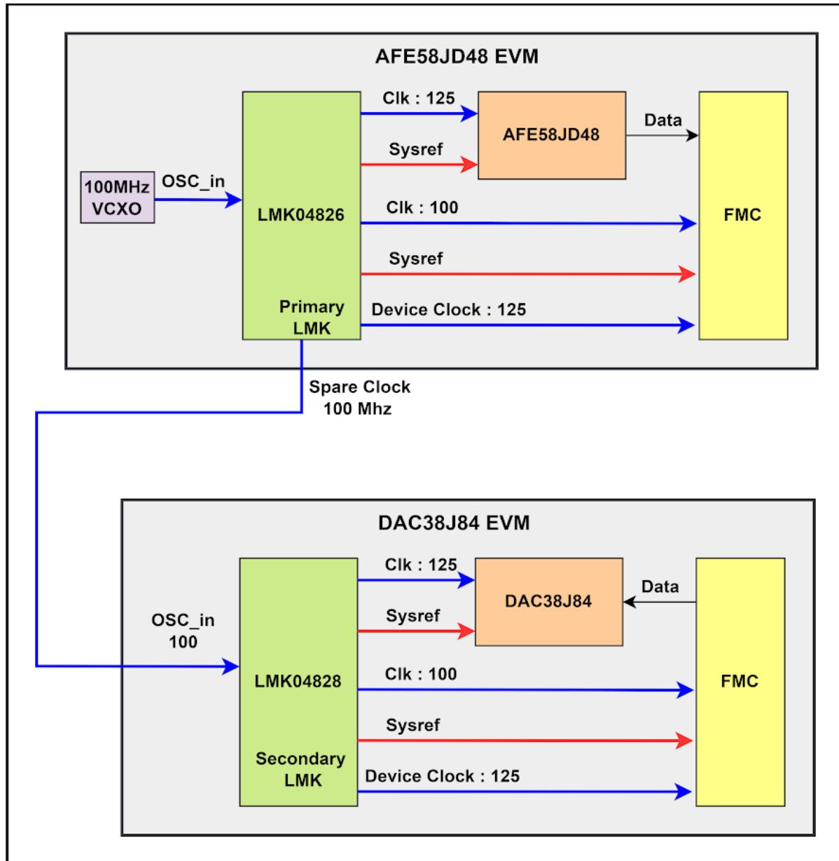
Figure 85. Clocking Structure for JESD204B Transmitter testing with DAC at 5 Gbps Line Rate (Here the oscillator input to the DAC LMK is ADC LMK clock output)
