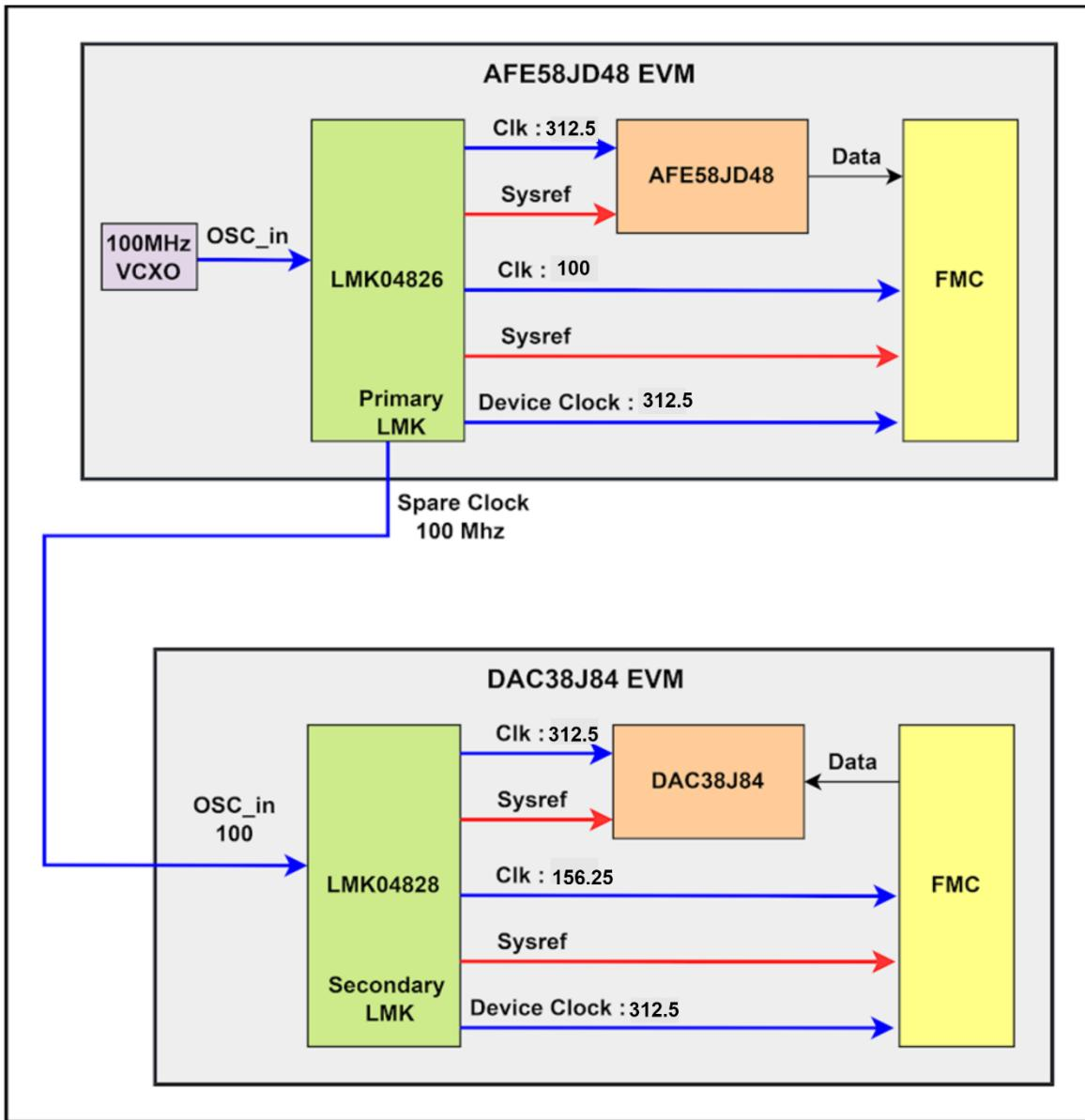
Figure 86: Clocking Structure for JESD204B Transmitter testing with DAC at 12.5 Gbps Line Rate (Here the oscillator input to the DAC LMK is ADC LMK clock output)
