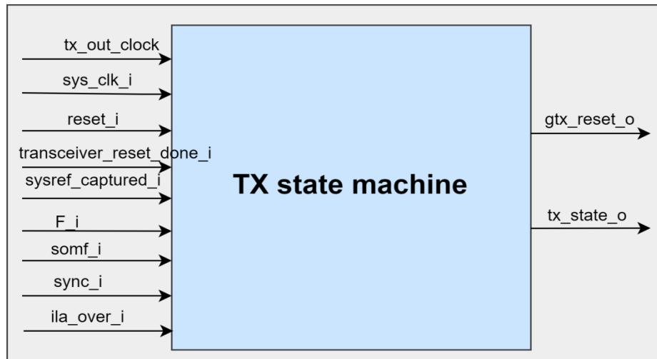
Figure 7.TX State machine Block design I/O signals
