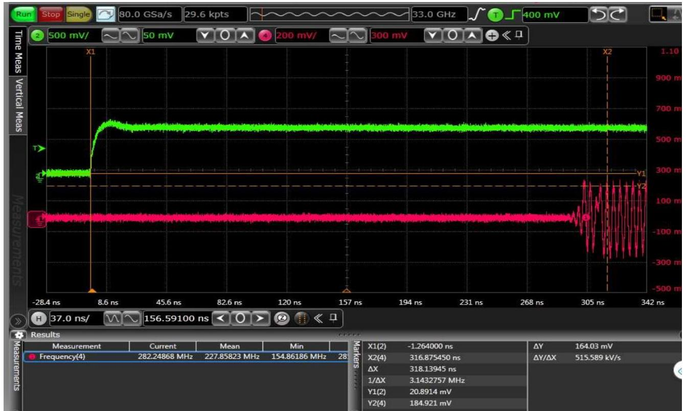
Figure 92: DAC Channel B output waveform at 12.5 Gbps Line Rate
