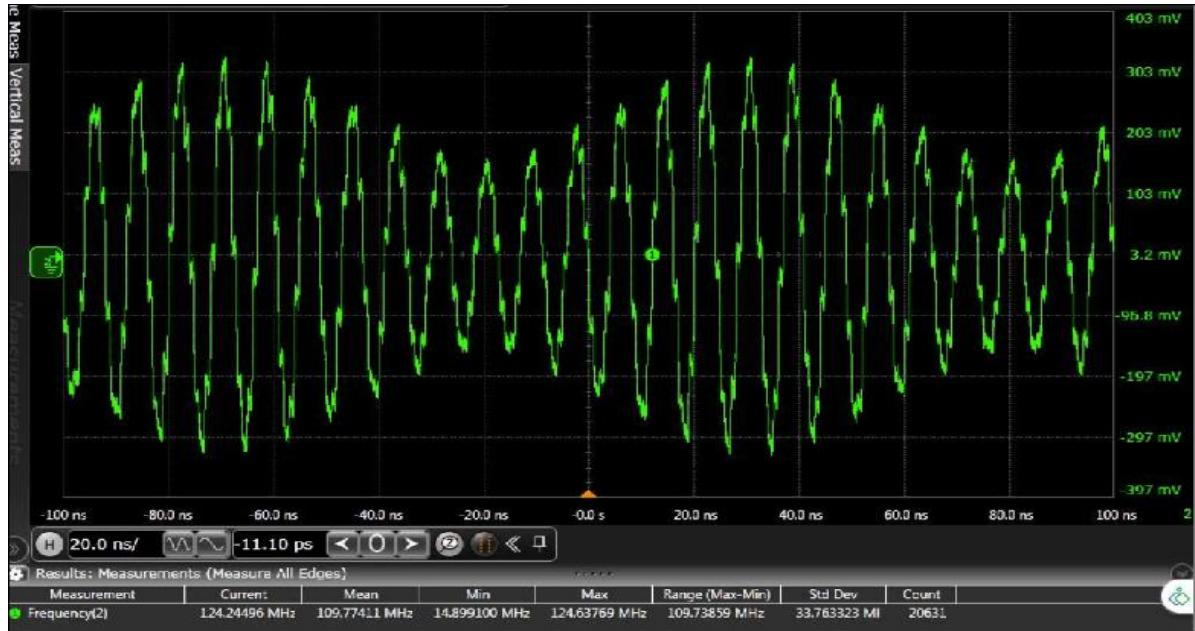
Figure 56.TC2: Time domain 120 MHz output waveform for x4 interpolation, LMF = 442 mode
