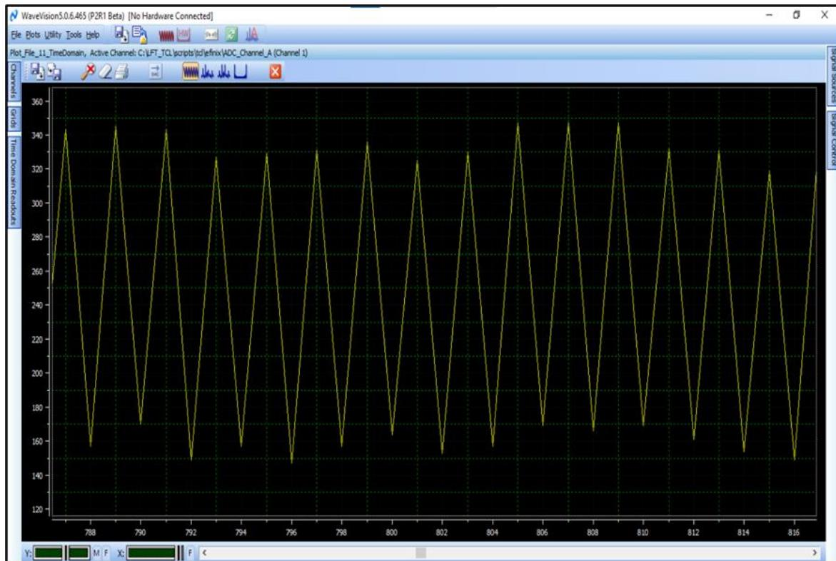
Figure 111.TC 0: Time domain plot for captured waveform for input frequency of 62.5 MHz
