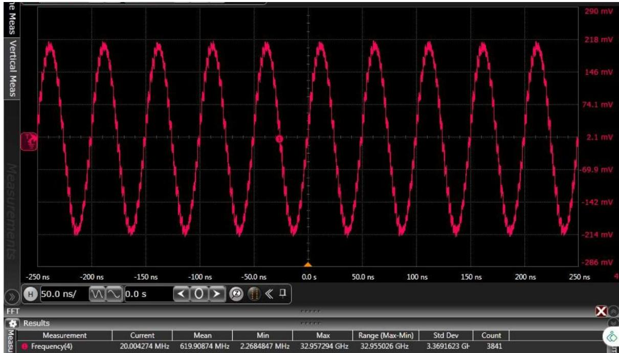
Figure 64. TC4 : Time domain 20 MHz output waveform for x4 interpolation, LMF = 244 mode
