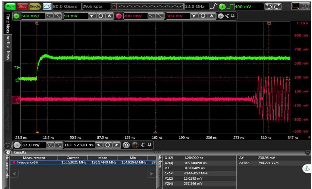
Figure 93: DAC Channel C output waveform at 12.5 Gbps Line Rate
