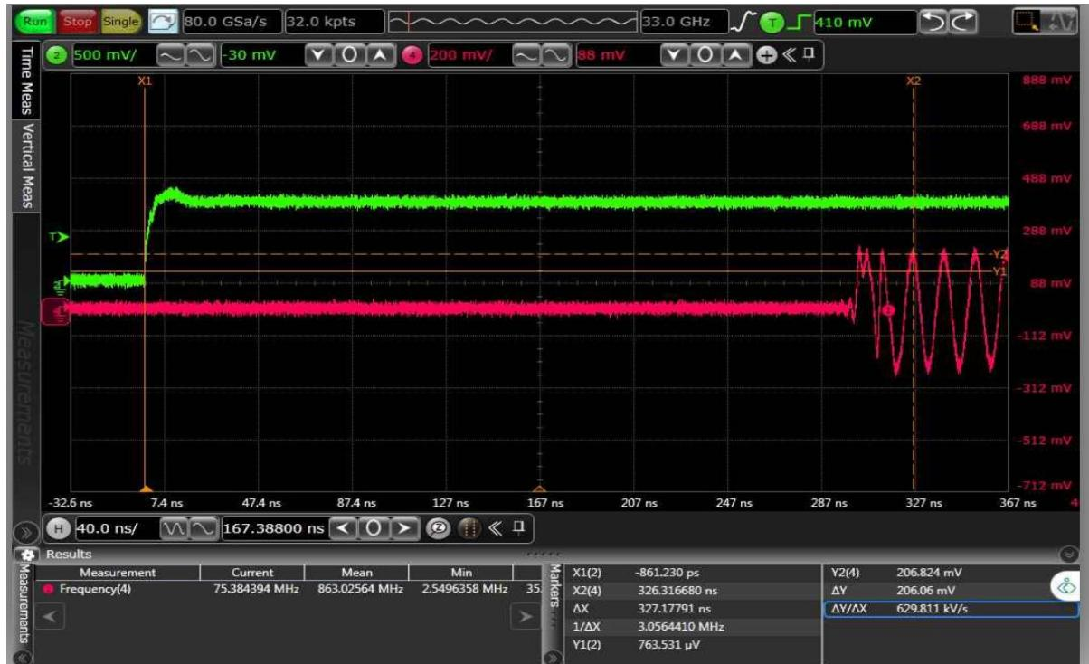
Figure 90: Deterministic Latency Delay of 327.17 ns without Heat Sink for input waveform of 75 MHz at 12.5 Gbps Line Rate
