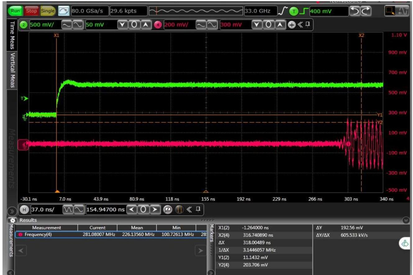
Figure 94: DAC Channel D output waveform at 12.5 Gbps Line Rate
