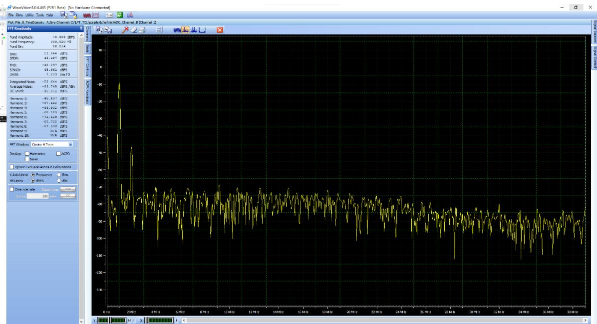
Figure 116.TC 0: Frequency domain plot for captured waveform for input frequency of 1 MHz
