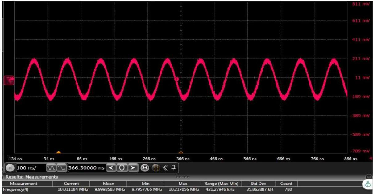
Figure 48.TC1: Time domain 10 MHz output waveform for x2 interpolation, LMF = 442 mode
