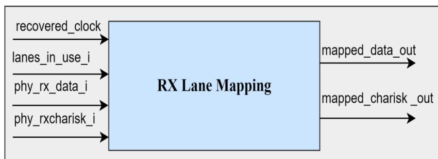
Figure 20. RX Lane Mapping I/O signals
