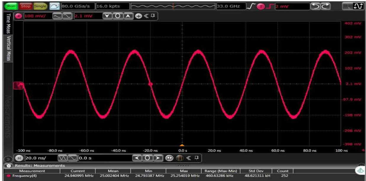
Figure 81: TC5: Time domain 25 MHz output waveform for x8 interpolation, LMF = 244 mode
