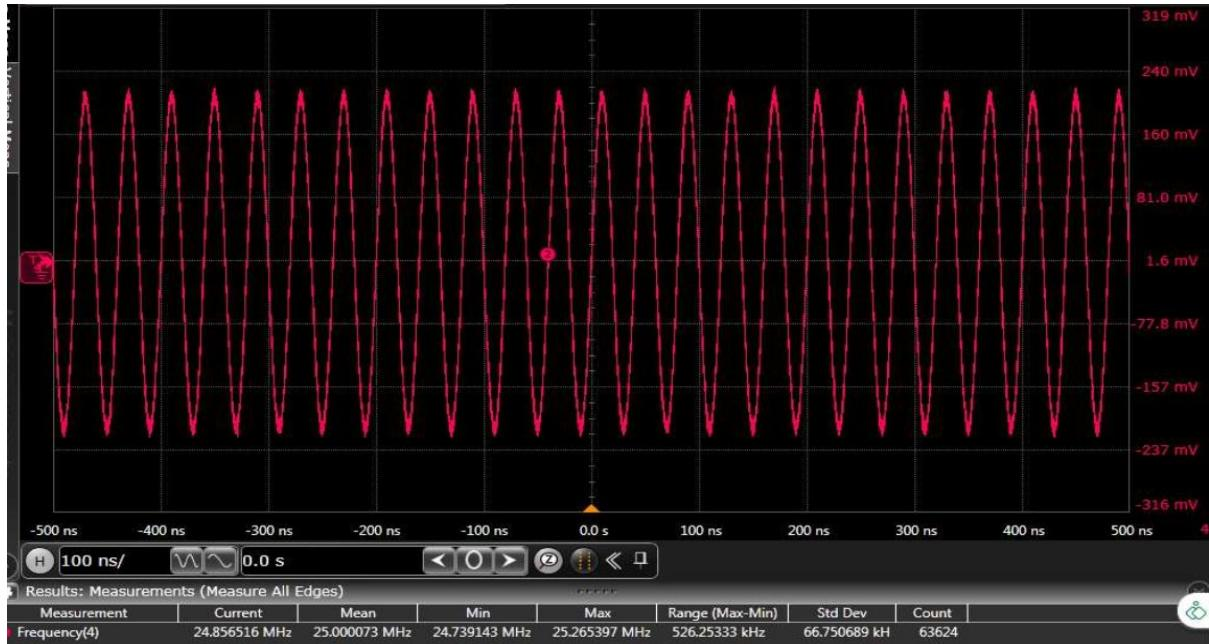
Figure 73.:TC2: Time domain 25 MHz output waveform for x4 interpolation, LMF = 442 mode
