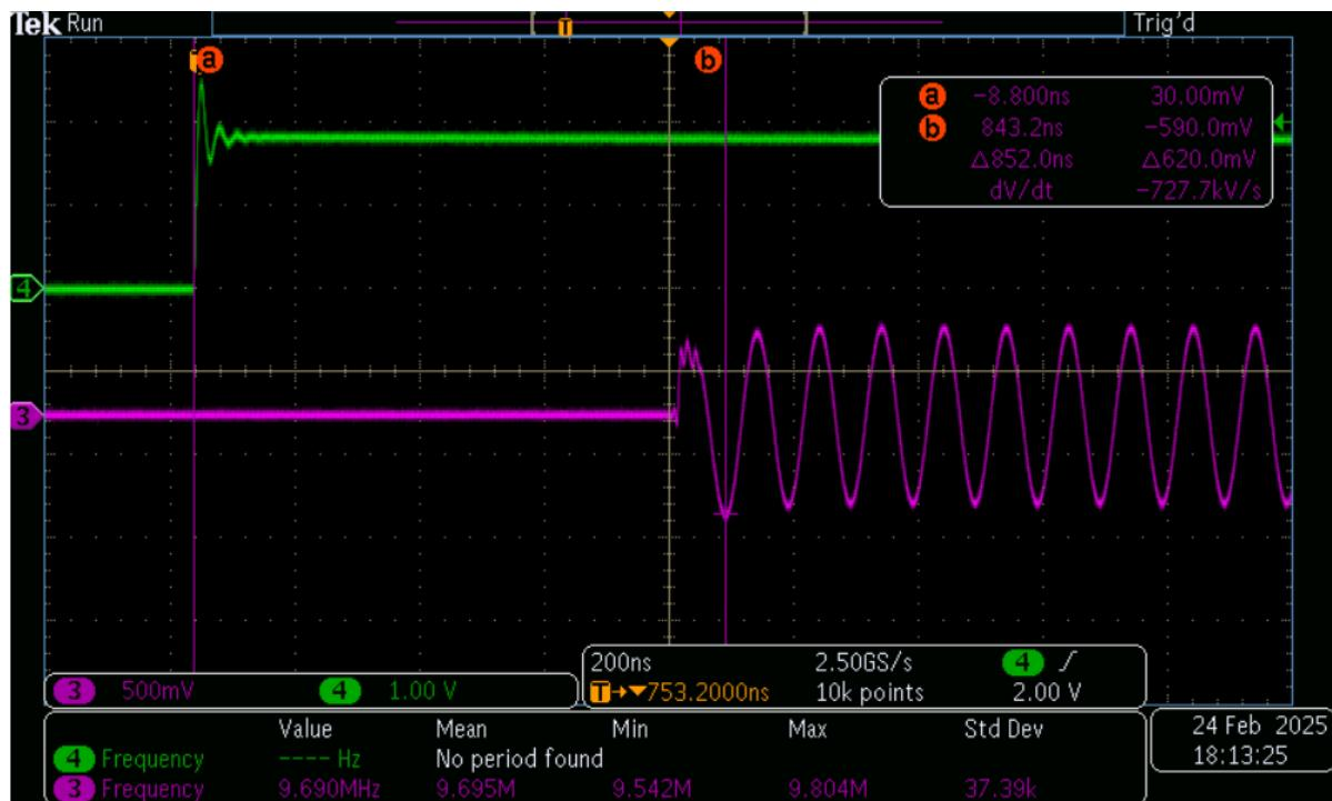
Figure 87.Deterministic Latency capture between trigger signal and DAC output at input frequency of 10MHz
