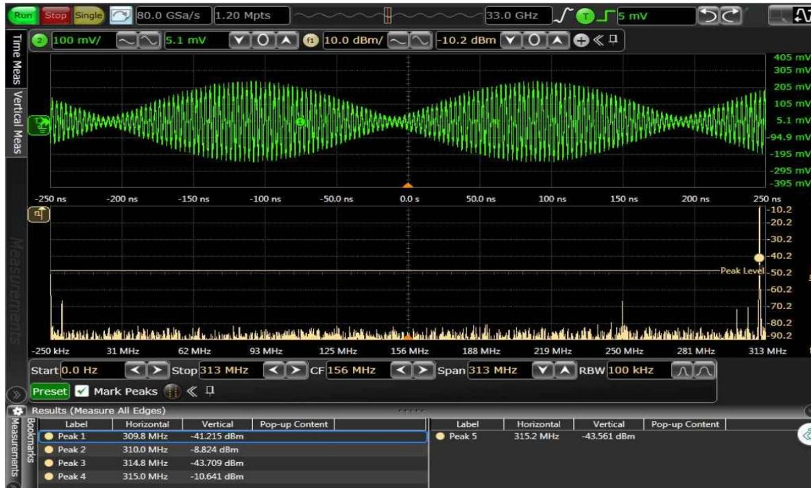
Figure 76:TC2: Time domain & Frequency Domain 310 MHz output waveform for x4 interpolation, LMF = 442 mode
