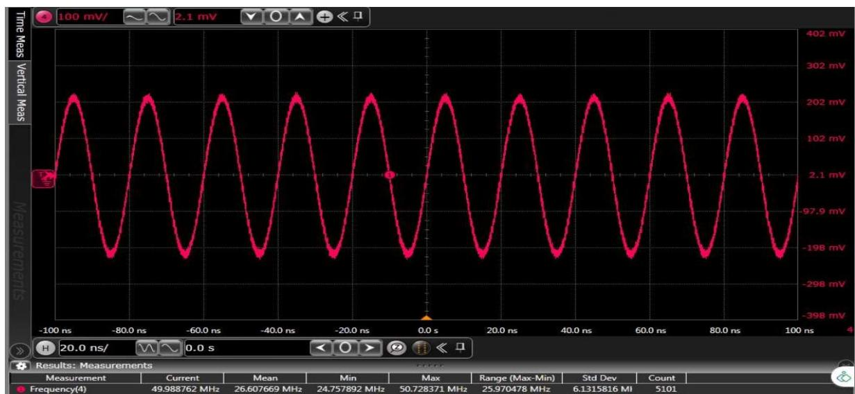
Figure 82: TC5: Time domain 50 MHz output waveform for x8 interpolation, LMF = 244 mode
