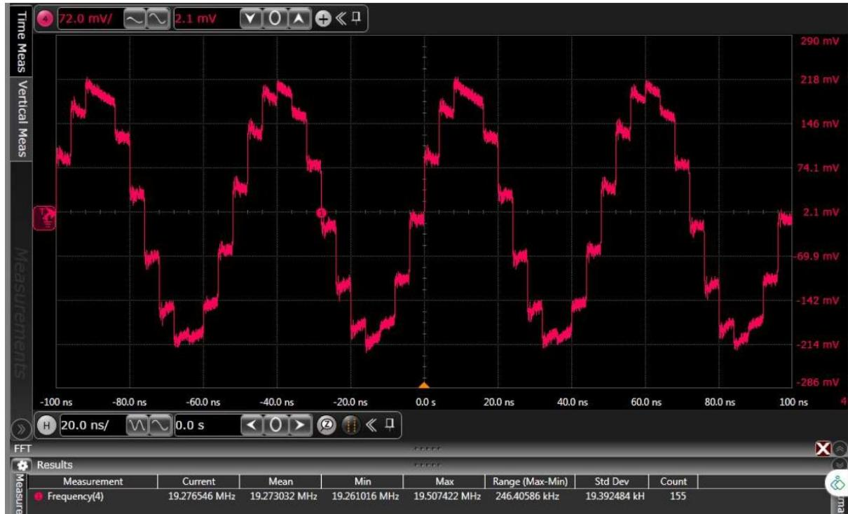
Figure 60.TC3: Time domain 20 MHz output waveform for x2 interpolation, LMF = 244 mode
