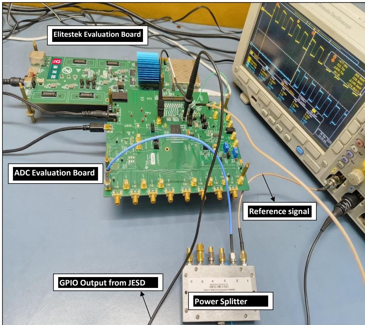
Figure 121. Test set up of Elitestek Evaluation Board with ADC for testing Deterministic Latency at 5Gbps
