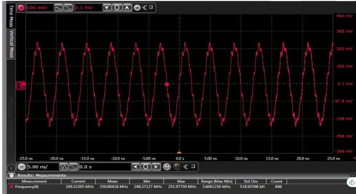
Figure 75:TC2: Time domain 250 MHz output waveform for x4 interpolation, LMF = 442 mode
