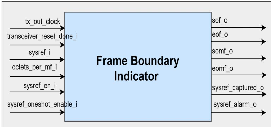
Figure 11. Frame Boundary Block
