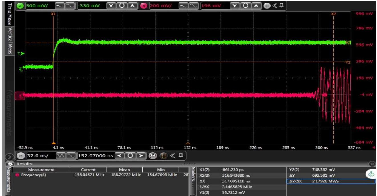
Figure 88.: Deterministic Latency capture between trigger signal and DAC output A at input frequency of 250MHz
