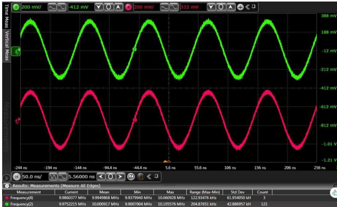
Figure 42. DAC output waveform for input frequency as 10MHz
