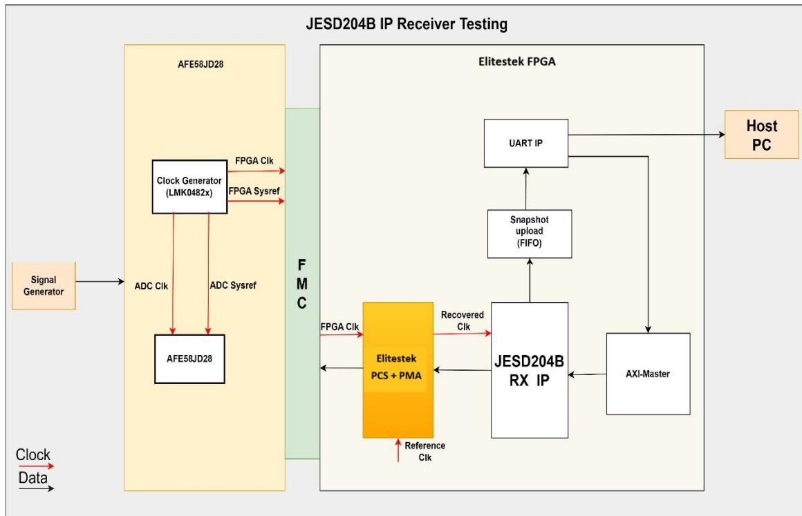
Figure 29.JESD204B IP Receiver Testing Block diagram
