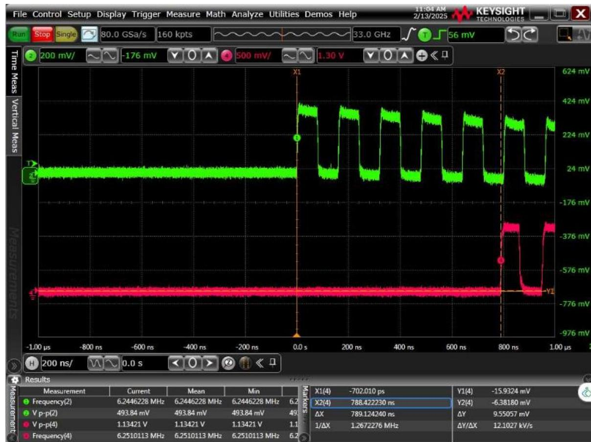
Figure 122. Deterministic Latency capture between input square and ADC MSB bit at input frequency of 6.25MHz
