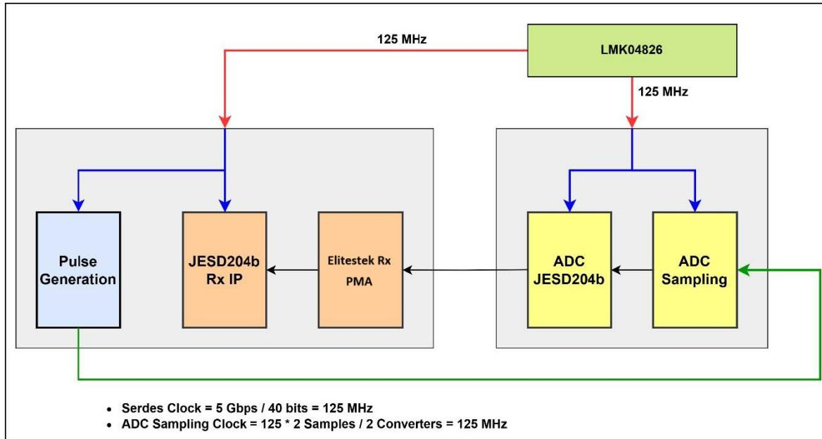
Figure 108 : Block Diagram depicting Clock Architecture for 5 Gbps Line Rate
