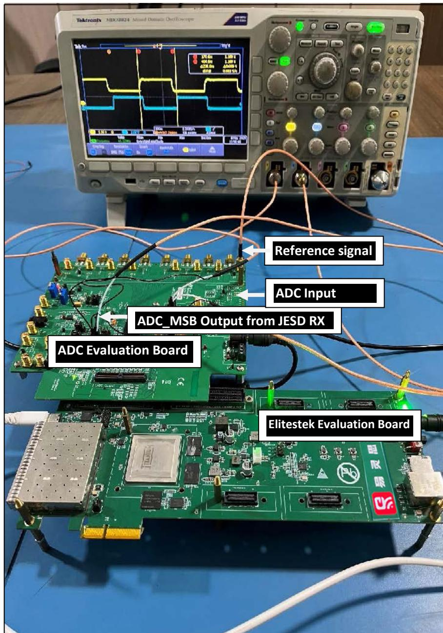
Figure 124. Test set up of Elitestek Evaluation Board with ADC for testing Deterministic Latency at 12.5Gbps
