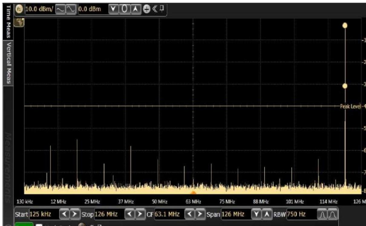
Figure 47.TCO: Frequency domain 120 MHz output waveform for x1 interpolation, LMF = 442 mode
