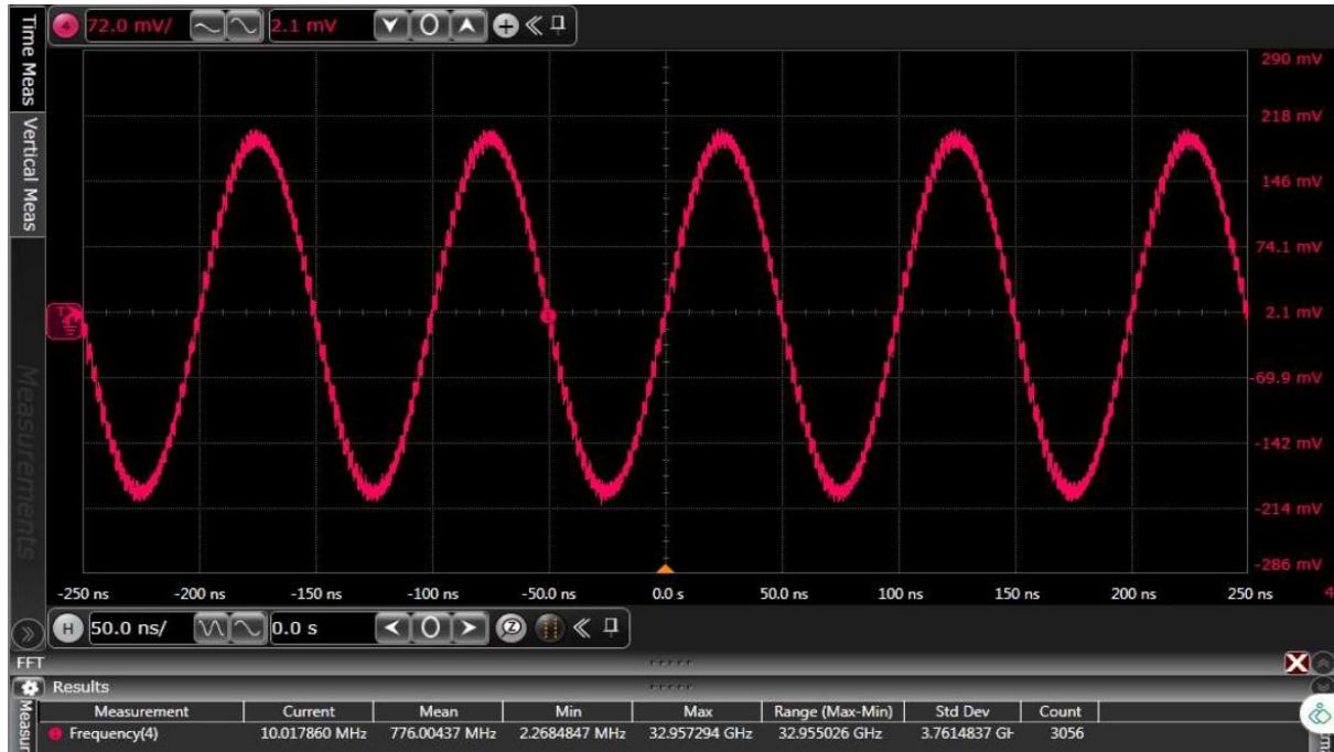
Figure 62.TC4: Time domain 10 MHz output waveform for x4 interpolation, LMF = 244 mode
