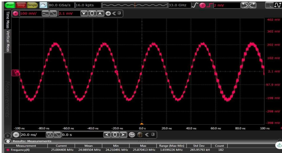
Figure 69:TC0: Time domain 25 MHz output waveform for x1 interpolation, LMF = 442 mode
