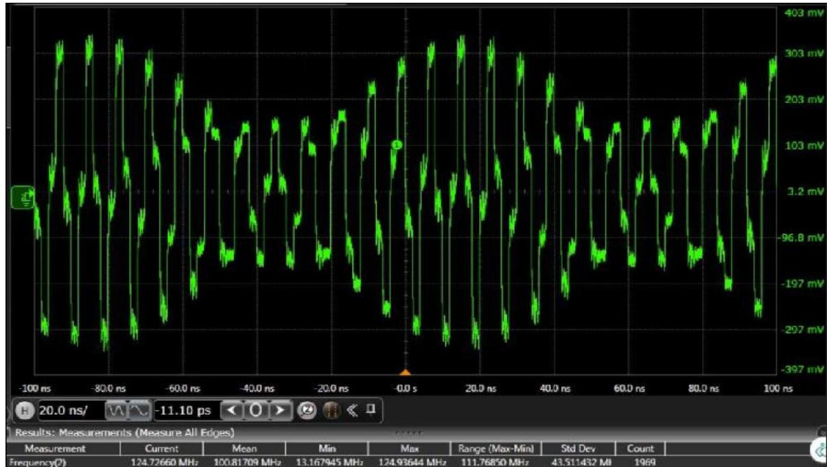
Figure 52.TC1: Time domain 120 MHz output waveform for x2 interpolation, LMF = 442 mode
