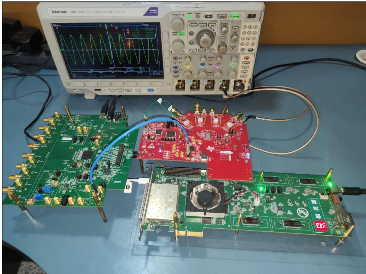
Figure 34. Test Setup of Elitestek Evaluation Board with DAC
