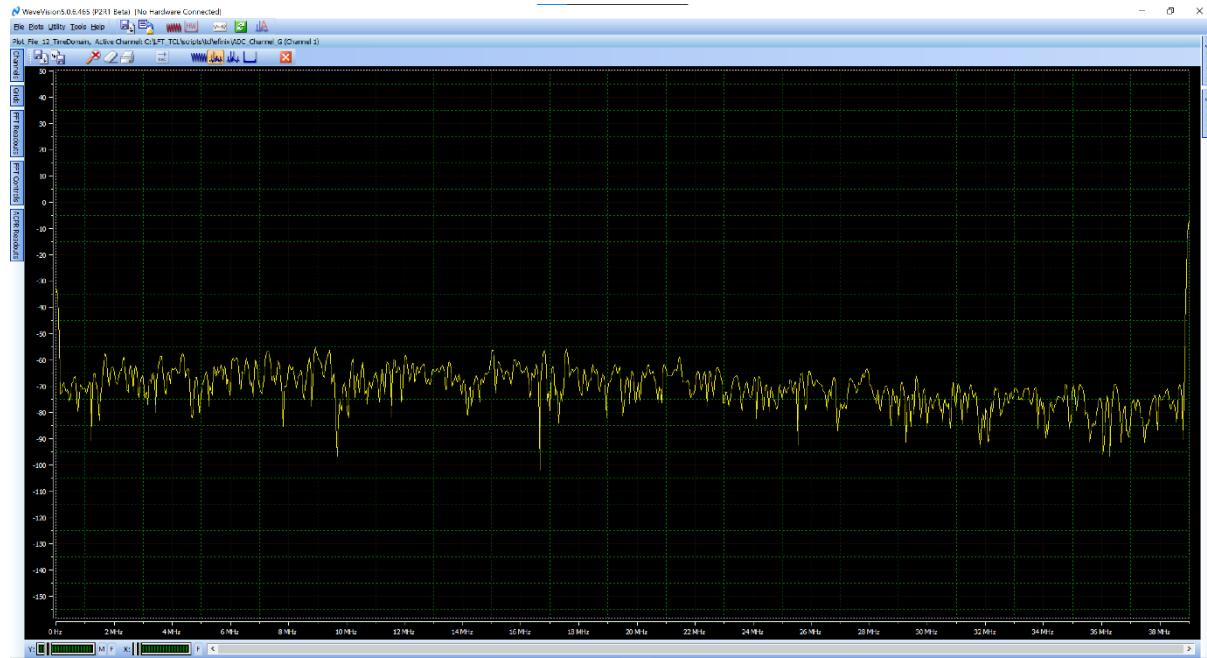
Figure 118.TC 0: frequency domain plot for captured waveform for input frequency of 39.0625 MHz
