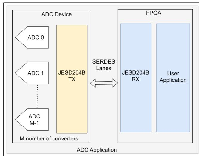
Figure 2. ADC Application Block Diagram
