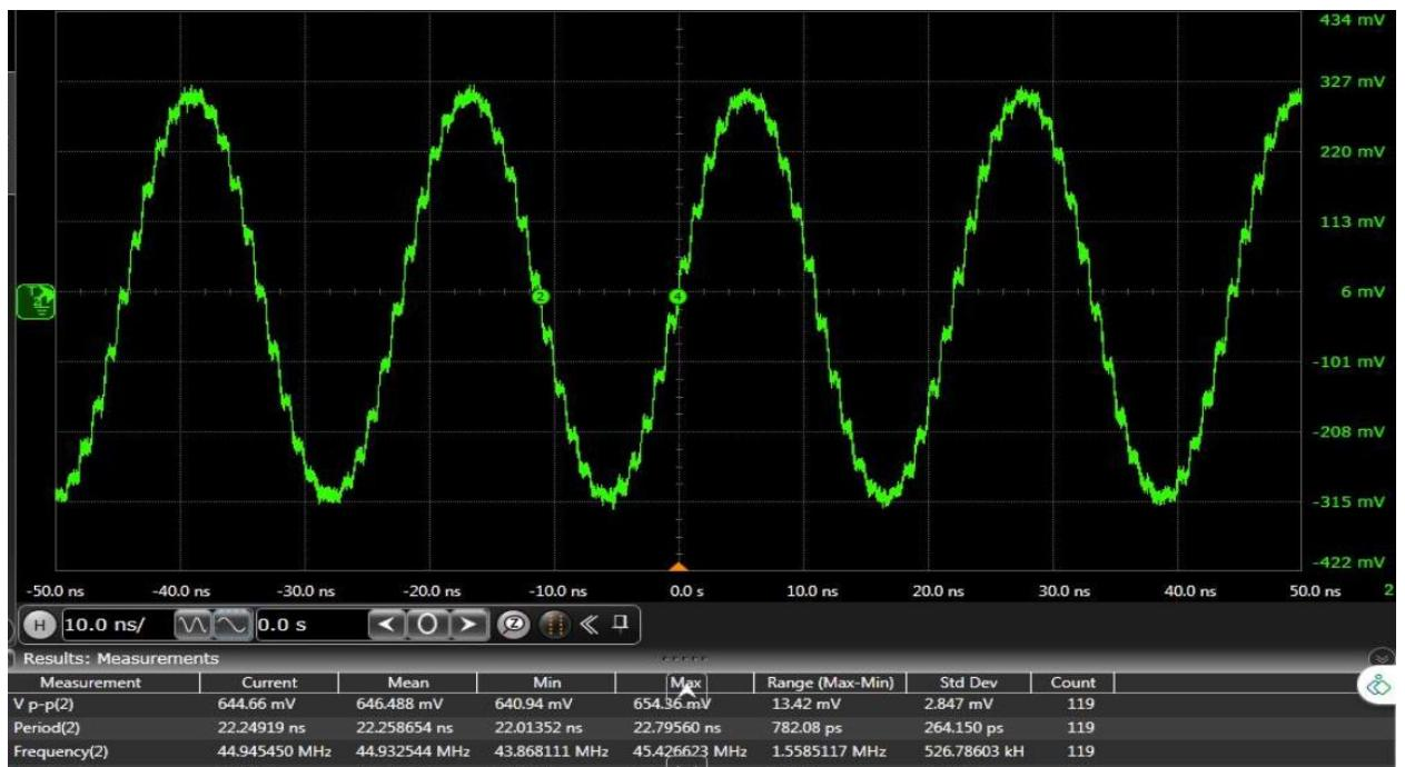
Figure 67. TC5: Time domain 20 MHz output waveform for x8 interpolation, LMF = 244 mode
