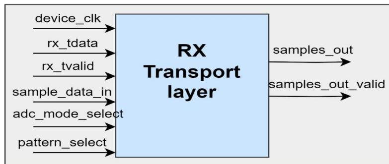
Figure 19. RX Transport layer I/O signals
