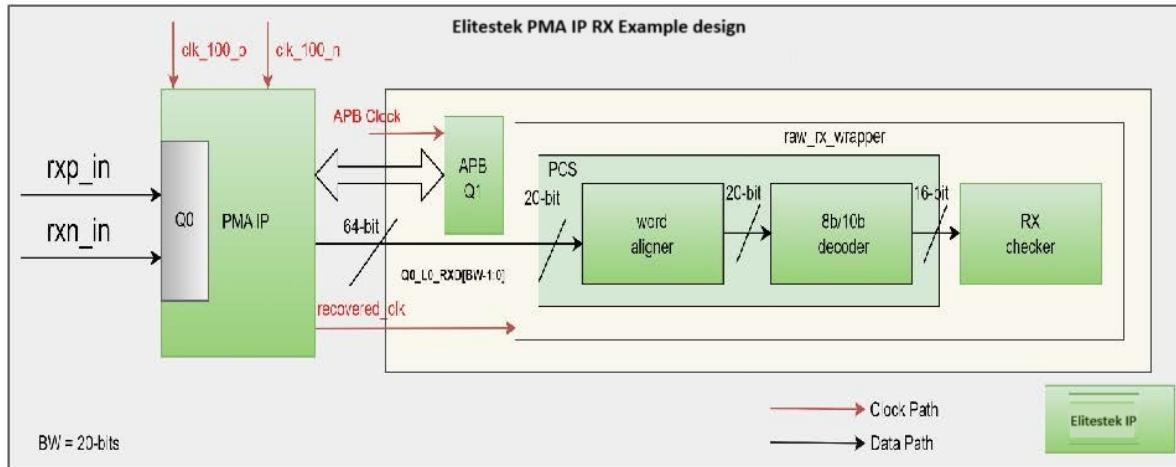
Figure 27. Elitestek PMA IP RX example design
