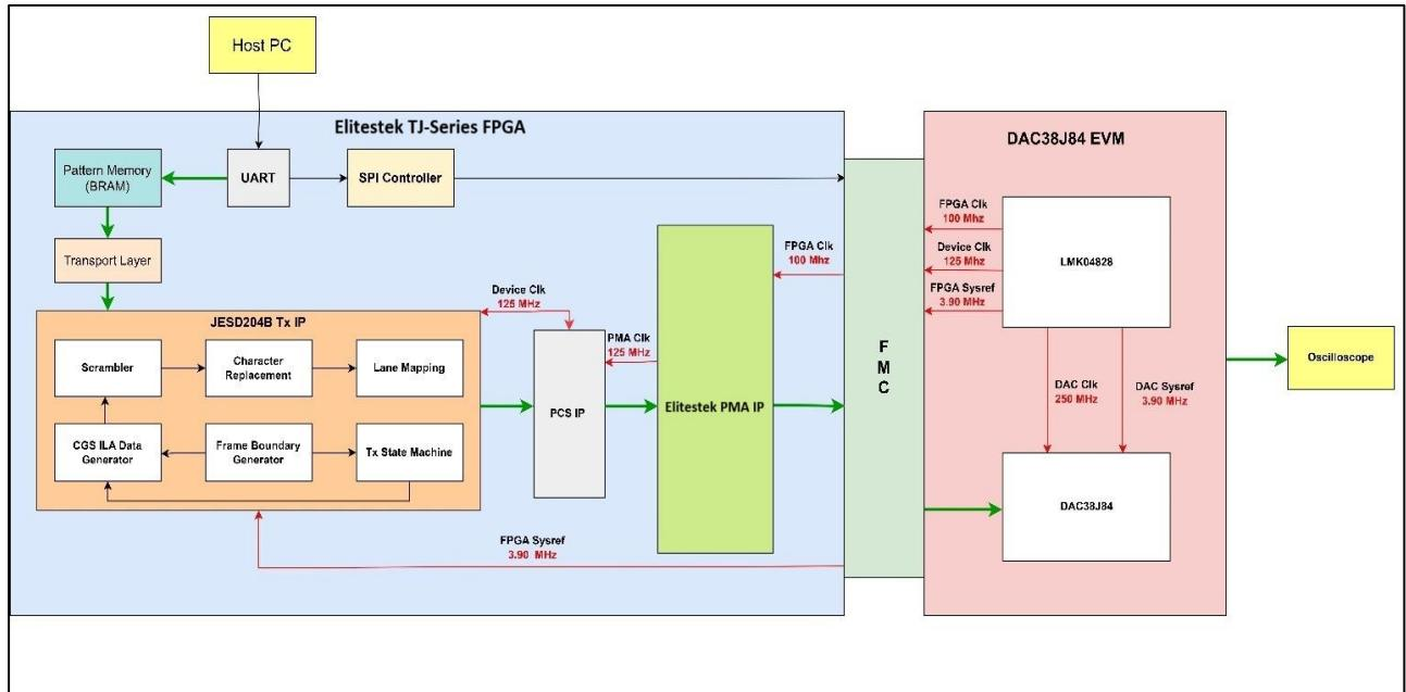
Figure 32. Hardware Validation Block Diagram of JESD204B Transmitter with DAC38J84 at 5 Gbps Line Rate
