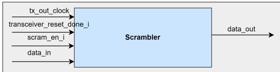
*Figure 12. Scrambler module I/O signals*
