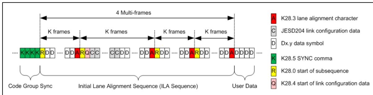
Figure 10. Initial Lane Alignment Sequence
