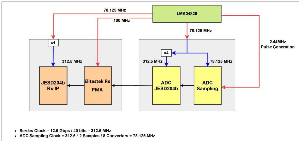
Figure 114: Block Diagram depicting Clock Architecture for 12.5 Gbps Line Rate
