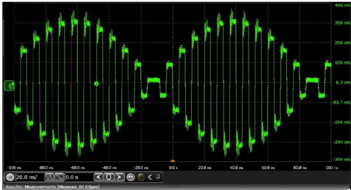
Figure 46.TCO: Time domain 120 MHz output waveform for x1 interpolation, LMF = 442 mode
