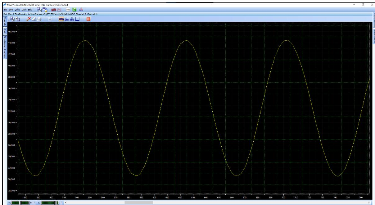
Figure 115 .TC 0: Time domain plot for captured waveform for input frequency of 1 MHz
