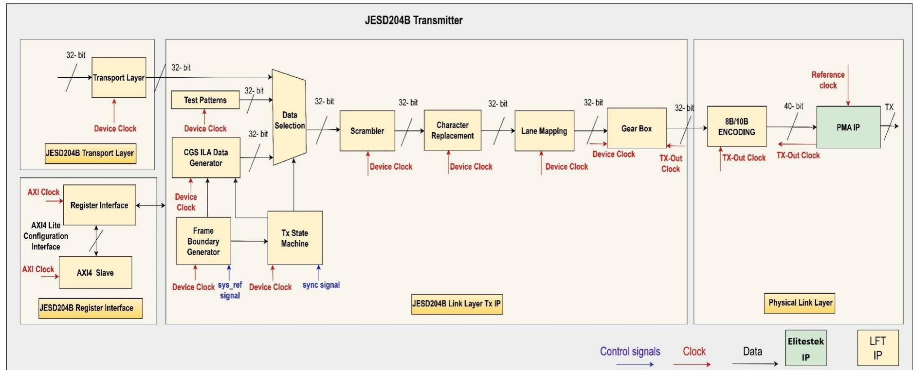
Figure 4. JESD204B Transmitter Block Diagram
