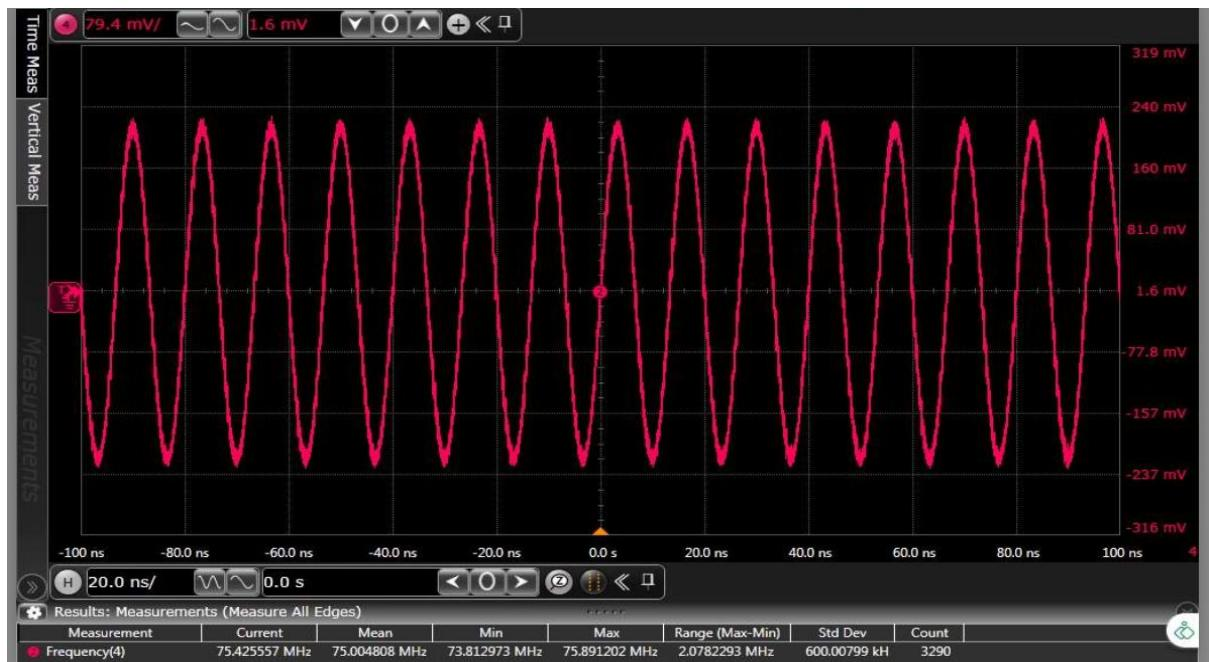
Figure 74:TC2: Time domain 75 MHz output waveform for x4 interpolation, LMF = 442 mode
