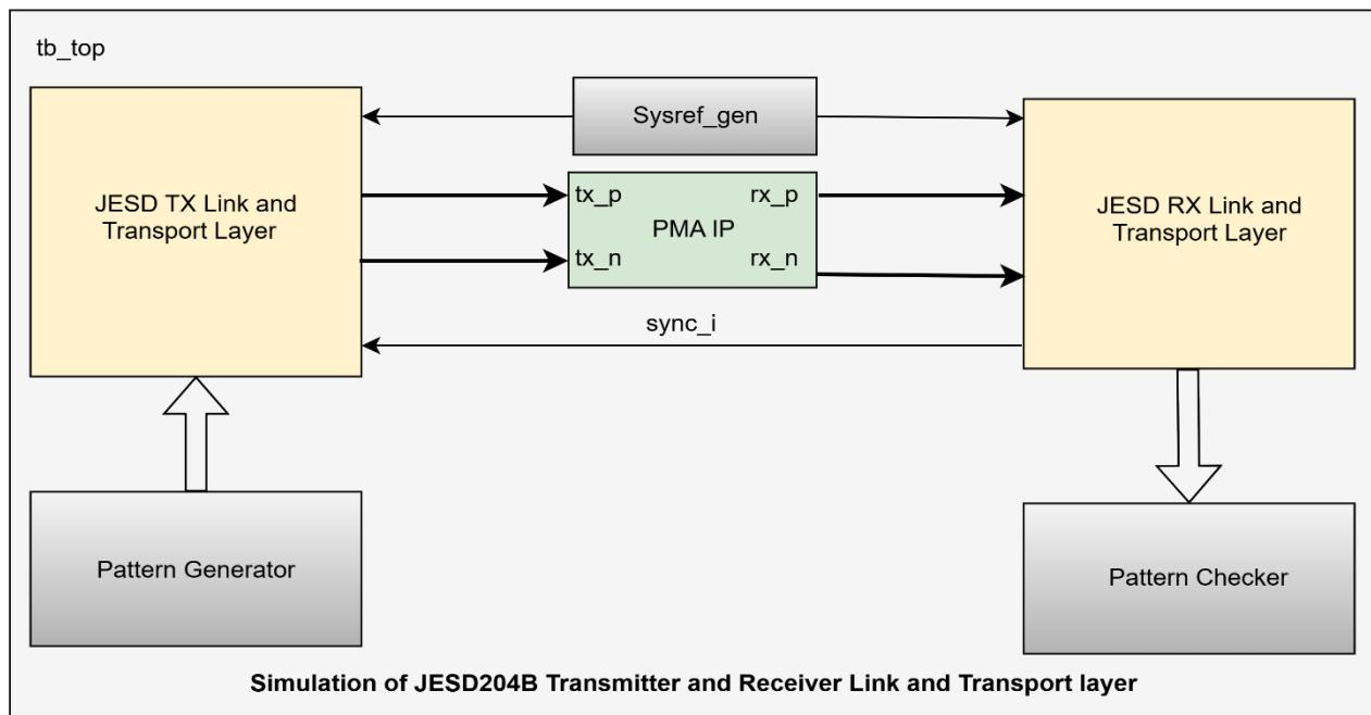
Figure 31. Simulation architecture for the JESD204B Link and Transport Layer
