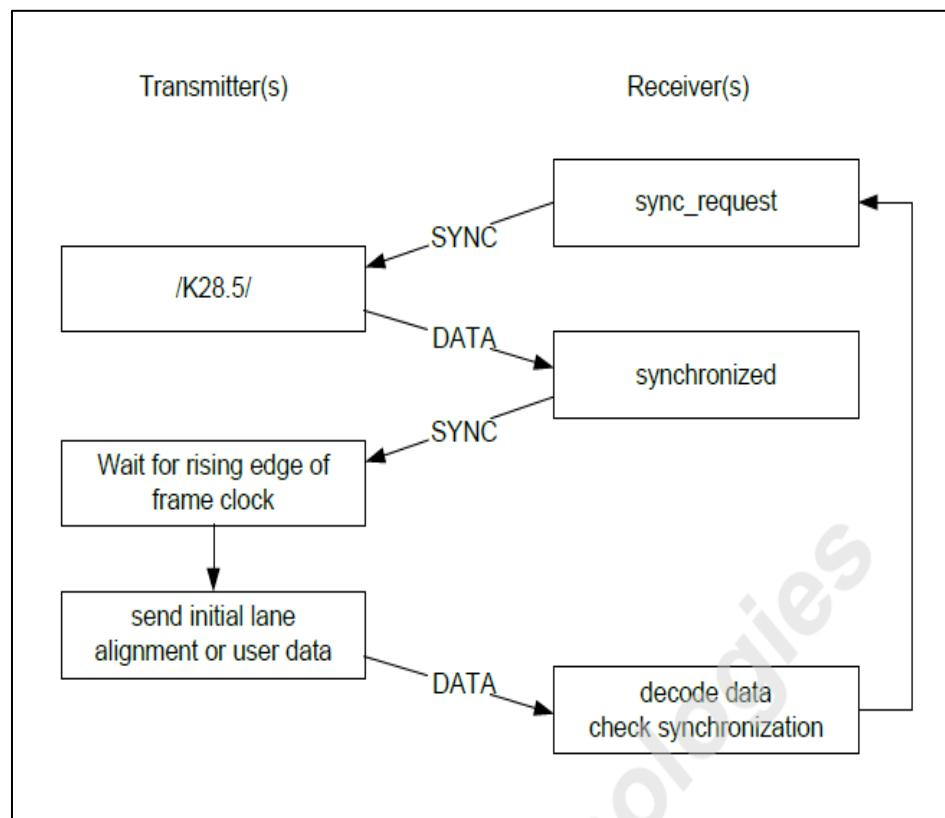
Figure 8. Synchronization process for Subclass 0
