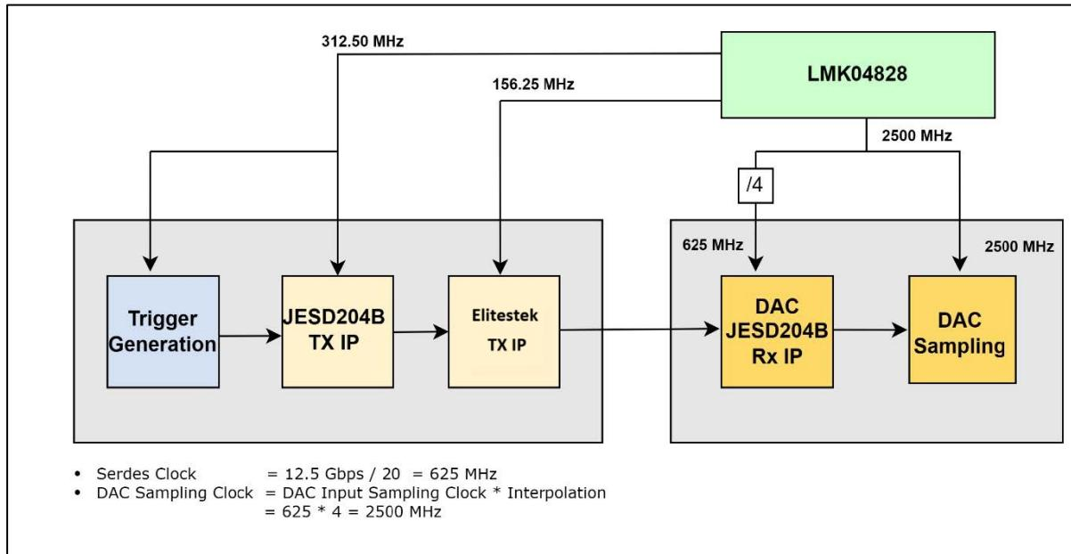
Figure 68: Block Diagram depicting Clocking Architecture for 12.5 Gbps
