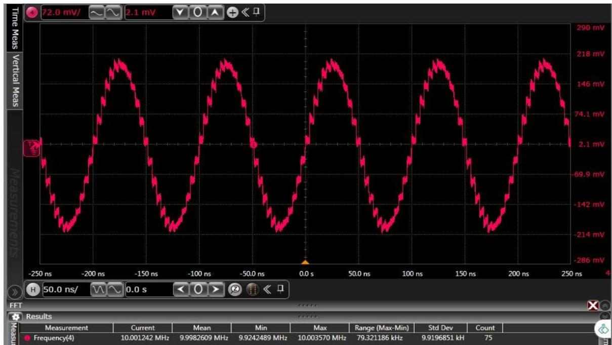
Figure 58.TC3: Time domain 10 MHz output waveform for x2 interpolation, LMF = 244 mode
