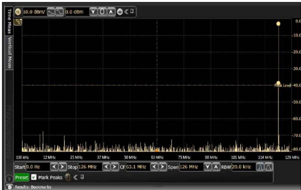
Figure 57.TC2: Frequency domain 120 MHz output waveform for x4 interpolation, LMF = 442 mode
