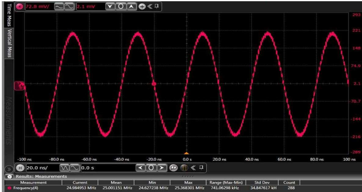
Figure 71. :TC1: Time domain 25 MHz output waveform for x2 interpolation, LMF = 442 mode
