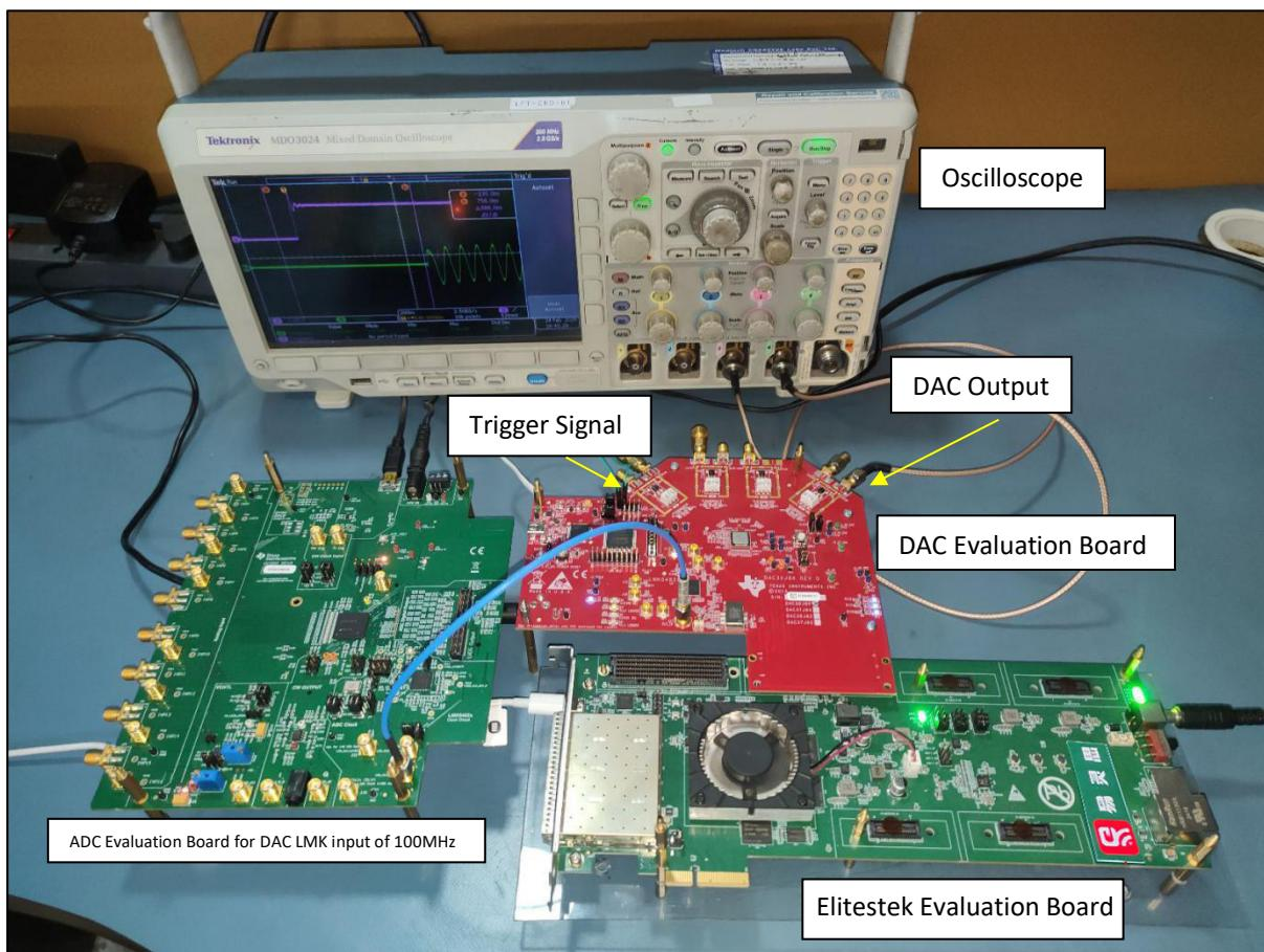
Figure 84. Test set up of Elitestek Evaluation Board with DAC for testing Deterministic Latency with external clock
