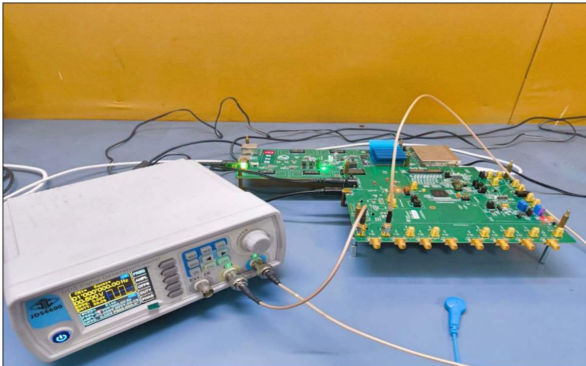
Figure 97. Test Set up of Elitestek Evaluation Board with ADC
