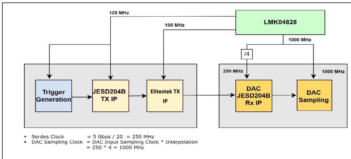
Figure 43: Block Diagram depicting Clock Architecture for 5 Gbps Line Rate
