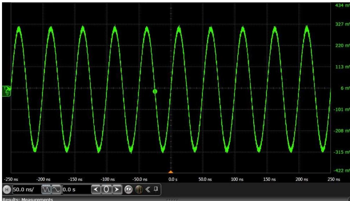
Figure 55.TC2 : Time domain 20 MHz output waveform for x4 interpolation, LMF = 442 mode
