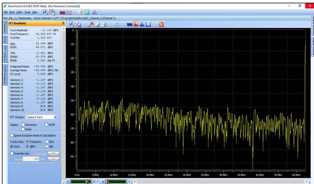
Figure 112.TC 0: frequency domain plot for captured waveform for input frequency of 62.5 MHz
