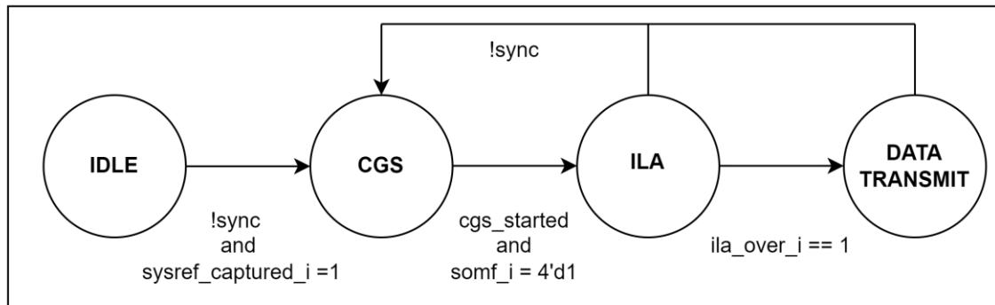
Figure 6.TX Data phase state machine
