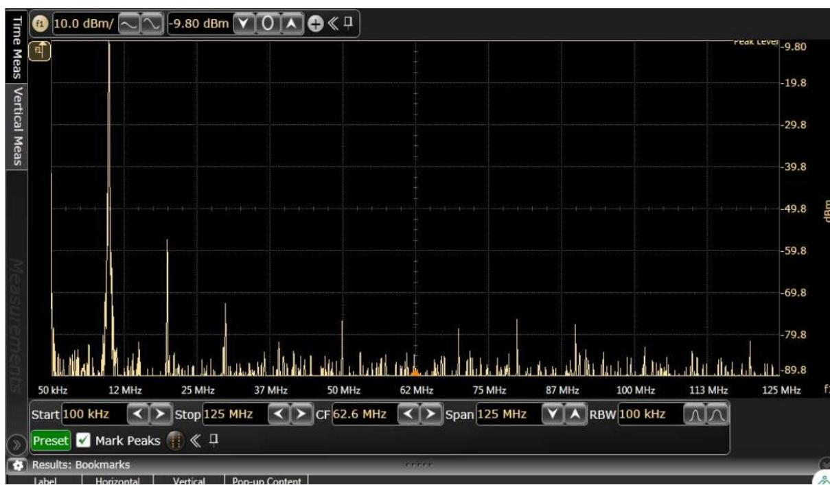
Figure 59.TC3: Frequency domain 10 MHz output waveform for x2 interpolation, LMF = 244 mode
