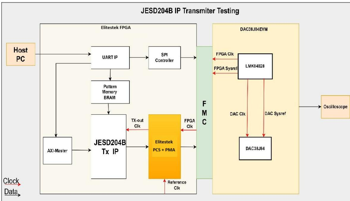
Figure 17. JESD204B IP Transmitter Testing Block diagram
