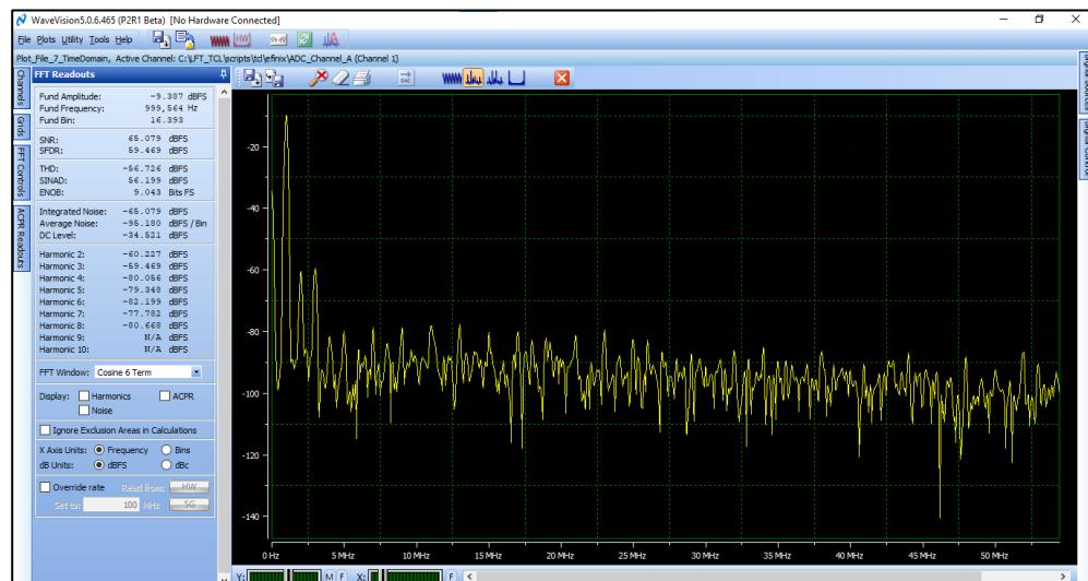
Figure 106. Frequency domain plot in WaveVision software
