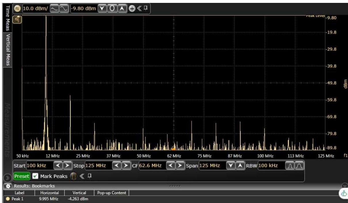
Figure 49.TC1: Frequency domain 10 MHz output waveform for x2 interpolation, LMF = 442 mode
