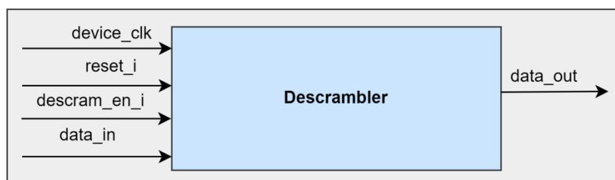
Figure 26. Descrambler Block I/O signals
