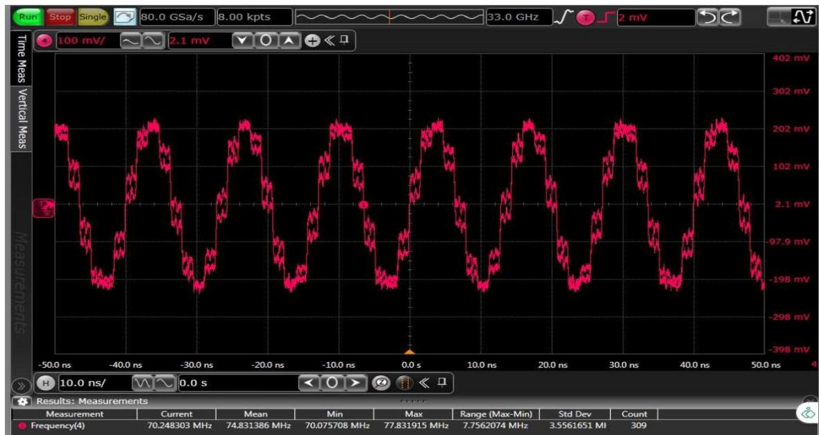
Figure 70.:TC0: Time domain 75 MHz output waveform for x1 interpolation, LMF = 442 mode
