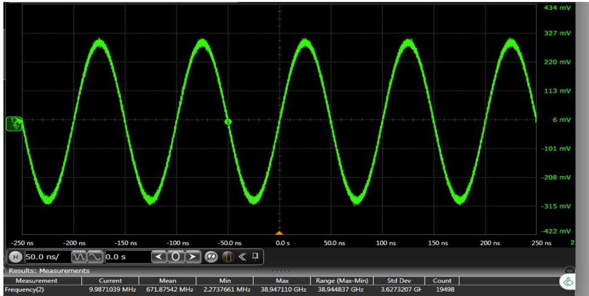
Figure 54.TC2 : Time domain 10 MHz output waveform for x4 interpolation, LMF = 442 mode
