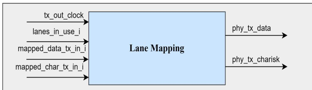
Figure 14. Lane Mapping I/O signals
