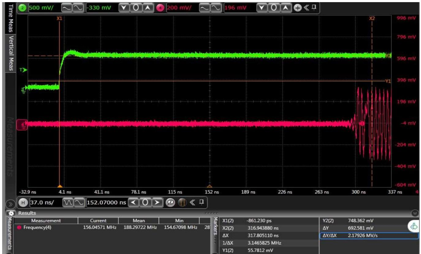
Figure 91: DAC Channel A output waveform at 12.5 Gbps Line Rate
