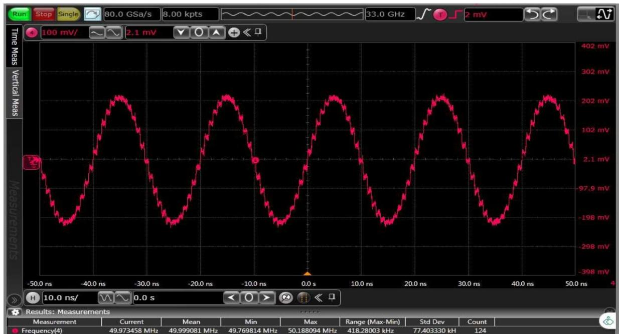
Figure 80: TC4: Time domain 50 MHz output waveform for x4 interpolation, LMF = 244 mode
