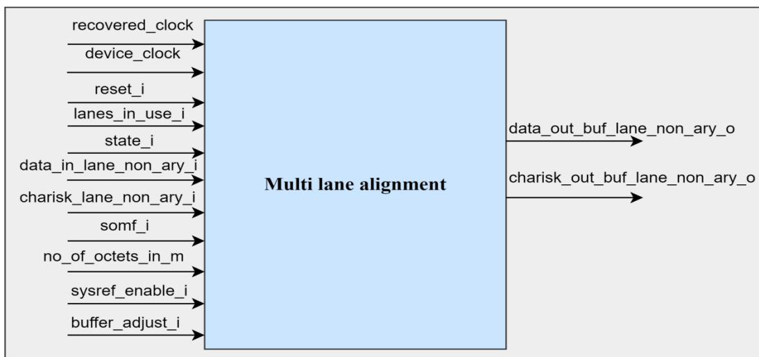
Figure 21. Multi lane alignment I/O signals
