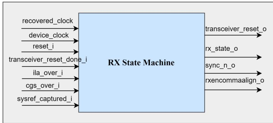
Figure 24. RX State Machine I/O signals
