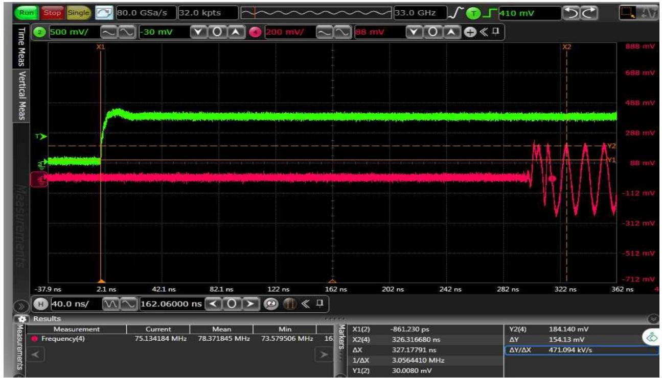
Figure 89: Deterministic Latency Delay of 327.17 ns with Heat Sink for input waveform of 75 MHz at 12.5 Gbps Line Rate
