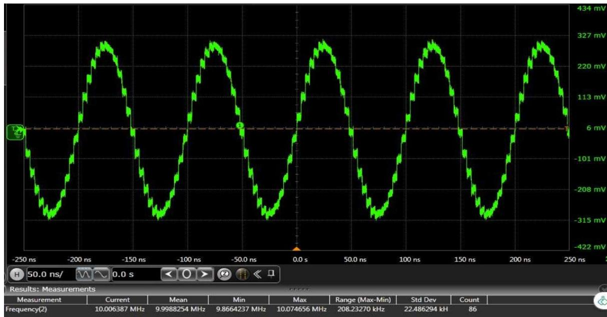
Figure 44. TCO : Time domain 10 MHz output waveform for x1 interpolation, LMF = 442 mode
