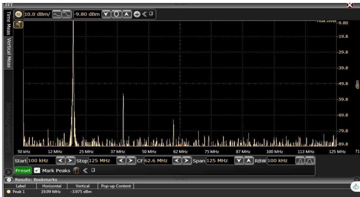
Figure 61.TC3: Frequency domain 20 MHz output waveform for x2 interpolation, LMF = 244 mode
