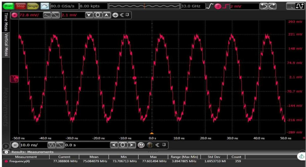
Figure 72. :TC1: Time domain 75 MHz output waveform for x2 interpolation, LMF = 442 mode
