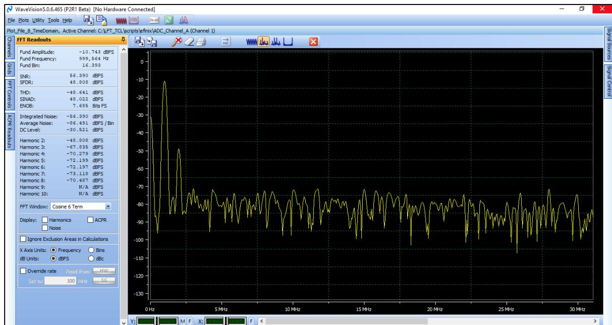
Figure 110.TC 0: Frequency domain plot for captured waveform for input frequency of 1 MHz
