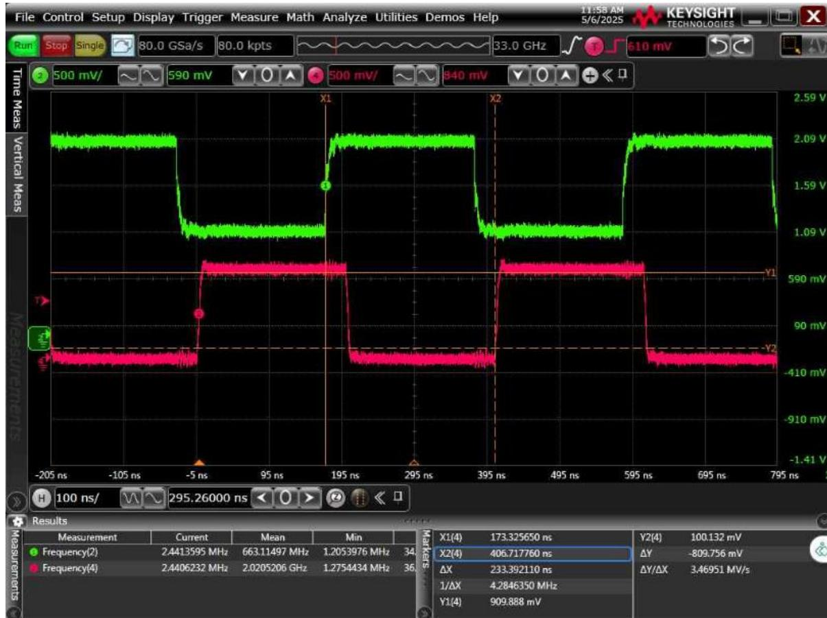
Figure 125. Deterministic Latency capture between input square and ADC MSB bit at input frequency of 2.44 MHz
