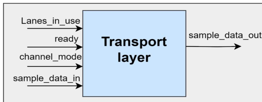
Figure 5. Transport layer Block design I/O signals
