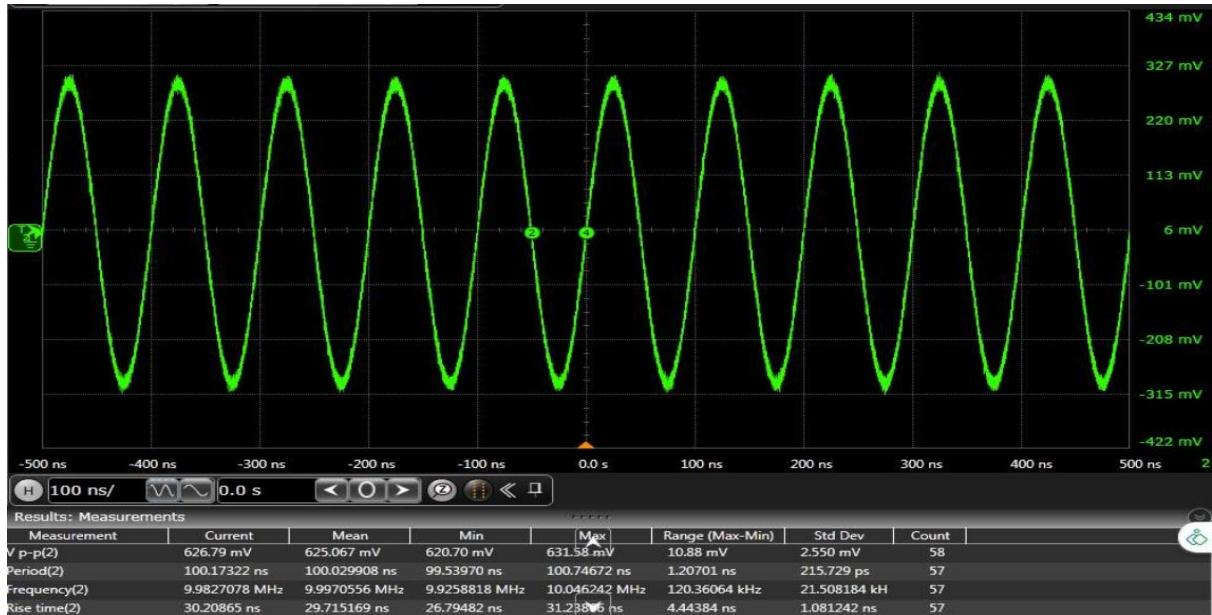
Figure 66.TC5: Time domain 10 MHz output waveform for x8 interpolation, LMF = 244 mode
