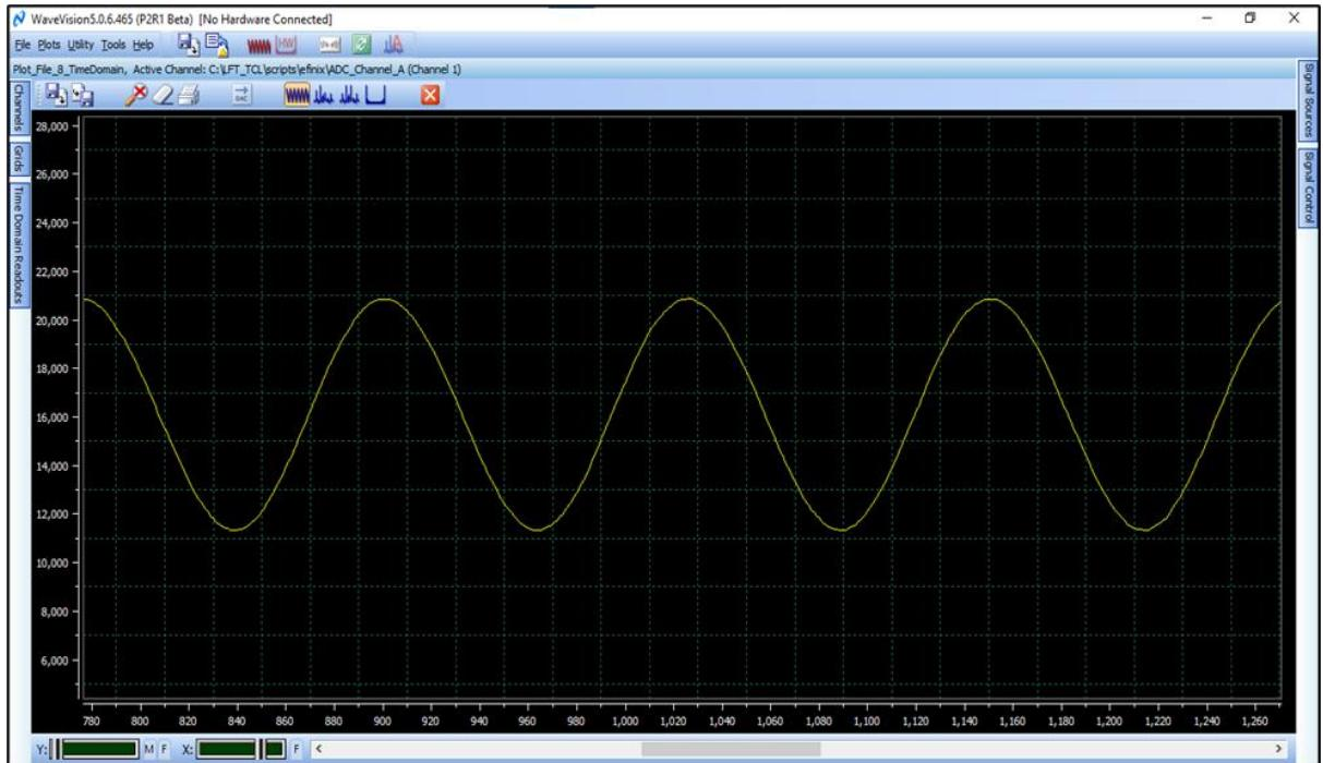
Figure 109 .TC 0: Time domain plot for captured waveform for input frequency of 1 MHz
