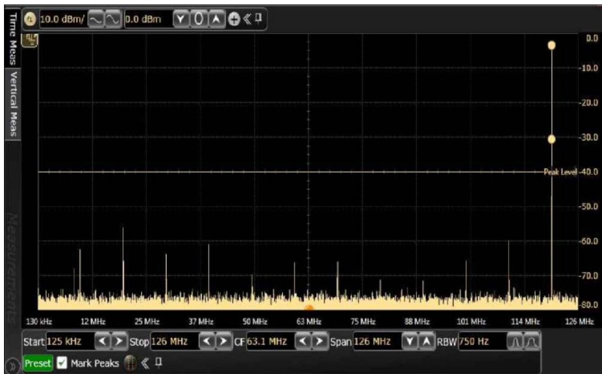
Figure 53.TC1: Frequency domain 120 MHz output waveform for x2 interpolation, LMF = 442 mode
