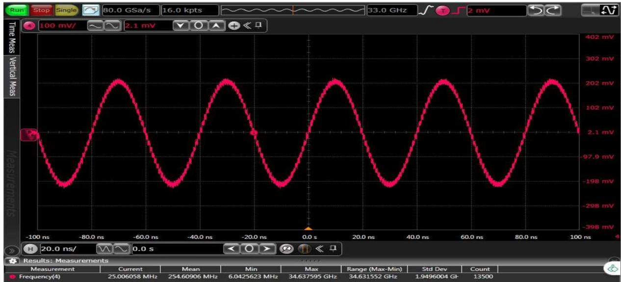
Figure 79: TC4: Time domain 25 MHz output waveform for x4 interpolation, LMF = 244 mode
