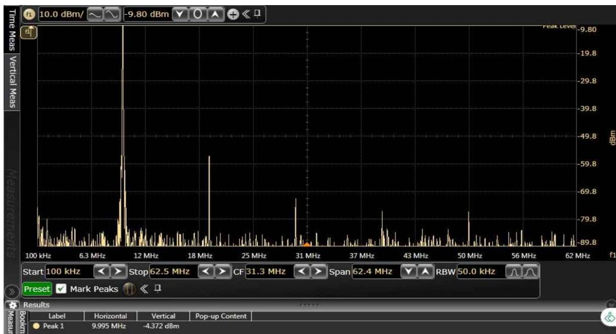
Figure 63.TC4 : Frequency domain 10 MHz output waveform for x4 interpolation, LMF = 244 mode
