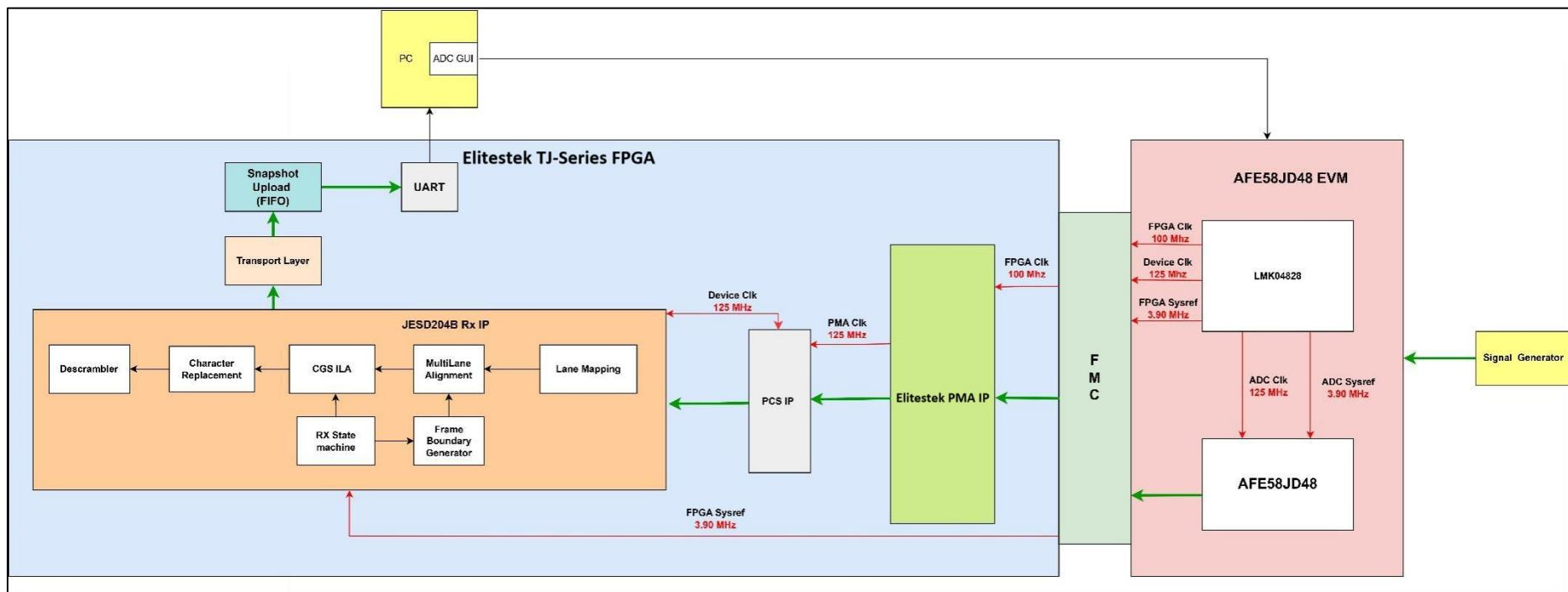
Figure 95. Hardware Validation Block Diagram of JESD204B Receiver with ADC AFE58JD48 at 5Gbps line rate
