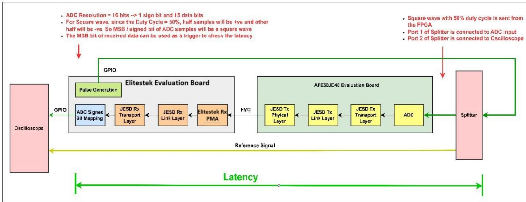
Figure 120. Deterministic Latency testing of JESD204B Receiver with ADC at 5Gbps
