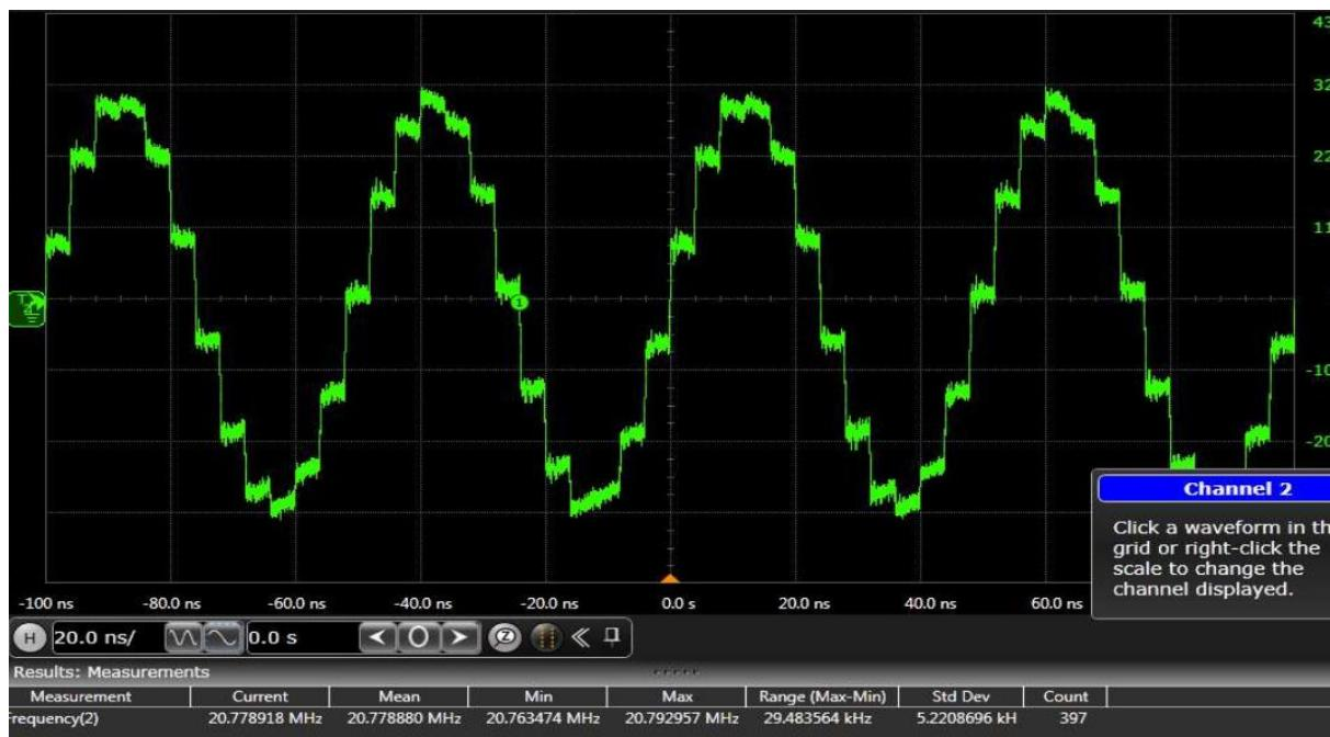
Figure 45.TCO: Time domain 20 MHz output waveform for x1 interpolation, LMF = 442 mode
