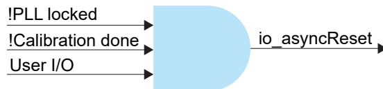
Figure 5: Gating SoC Reset
