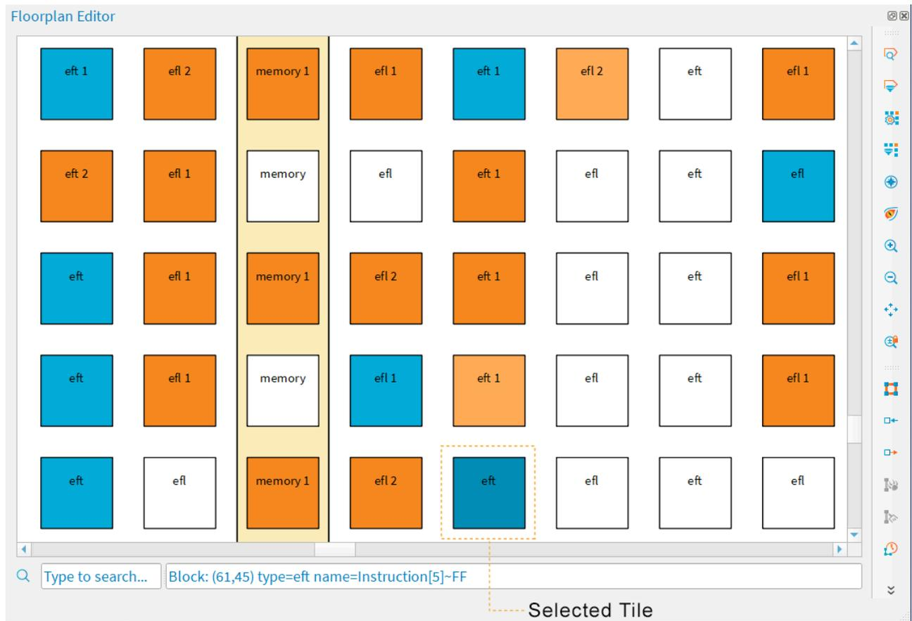
Notice that some tiles in the floorplan have a number. This number indicates how many routing lines are used in that tile. A tile used for logic (blue) can also be used as routing (indicated by the number). Orange means a tile is only used as routing.
