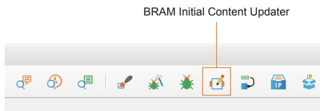
In the tool, you select the elaborated netlist memory that you want to update, not the post-map memory. Therefore, you do not need to know how synthesis decomposes and maps the memories to use this tool. Because this tool bypasses the full compilation flow, it does not update *<project>.map.v* and other intermediate compiler output files. As a result, the updated bitstream file will be out of sync with your other project files.
