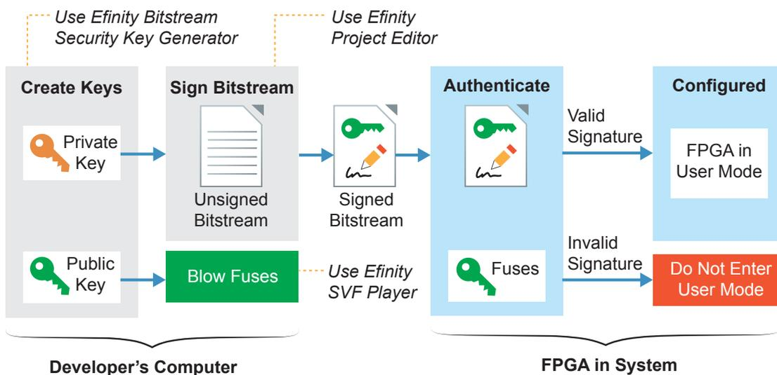
The public key is derived from the private key; the **.pem** is essentially a private/public key pair. The private key only exists in the **.pem**. The software uses it to sign the bitstream, but the bitstream and fuses only contain public key information. The FPGA uses the public key to validate the bitstream's signature; it cannot be used to re-sign a modified bitstream.
