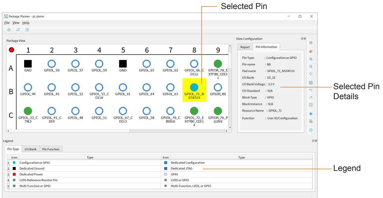
You can also hover over a pin for a quick view of the pin details.
