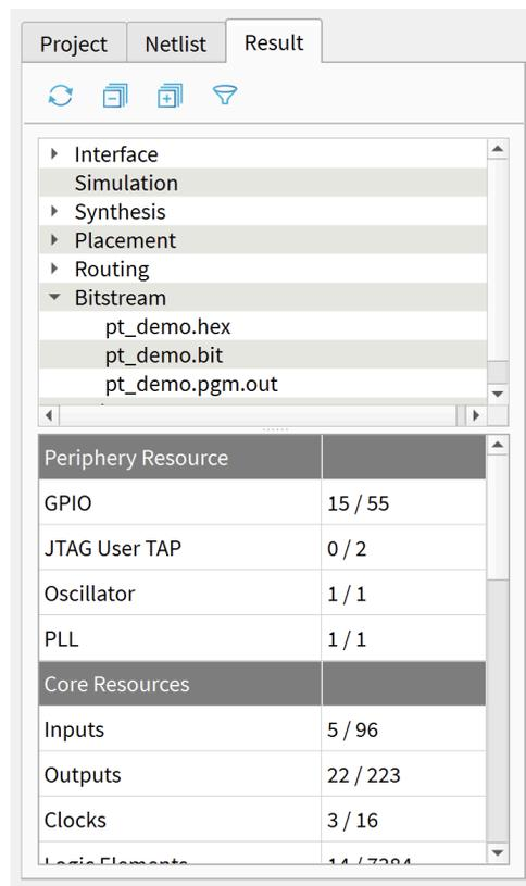
The numbers of inputs and outputs in the Core Resource section represent the connections between the core and the periphery; they are not package pins. See **<project>.place.rpt** on page 150 for more details.
